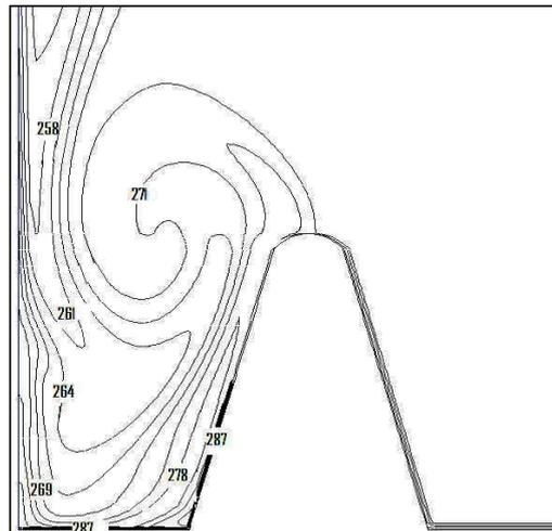
Fig. 7. temperature alignment line (K) after 12 minutes and 54 seconds of heat application.
