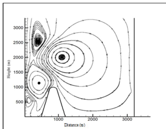
Fig. 8. flow lines after 12 minutes and 54 seconds of heat application.
