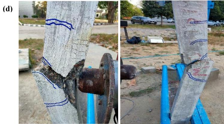
**Fig. 4.** Crack pattern of (a) M20 (b) M30 (c) M40 and (d) M50 concrete beam after impact
