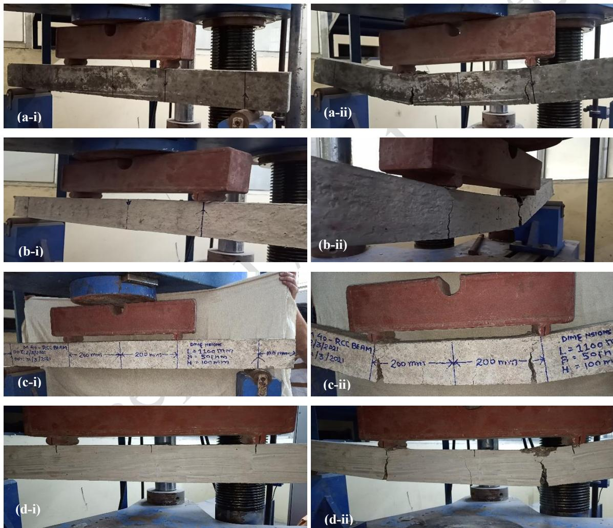
**Fig. 6.** Reinforced concrete beam of (a) M20 (b) M30 (c) M40 and (d) M50 concrete grades (i) before and (ii) after the four-point bending test
