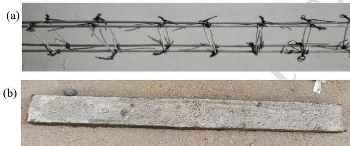
**Fig. 1.** (a) Reinforcement mesh and (b) concrete beam specimen
