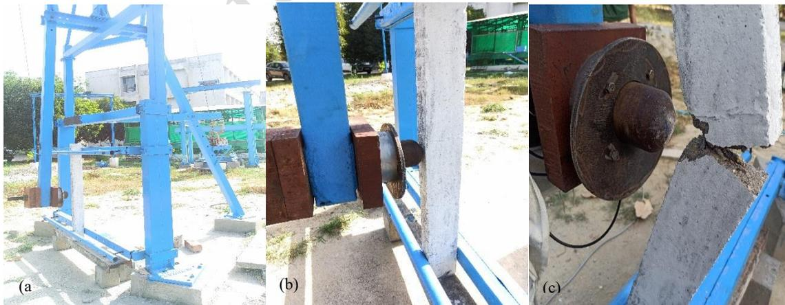
**Fig. 3.** (a) Testing frame (b) Impactor with load cell and (c) beam after impact
