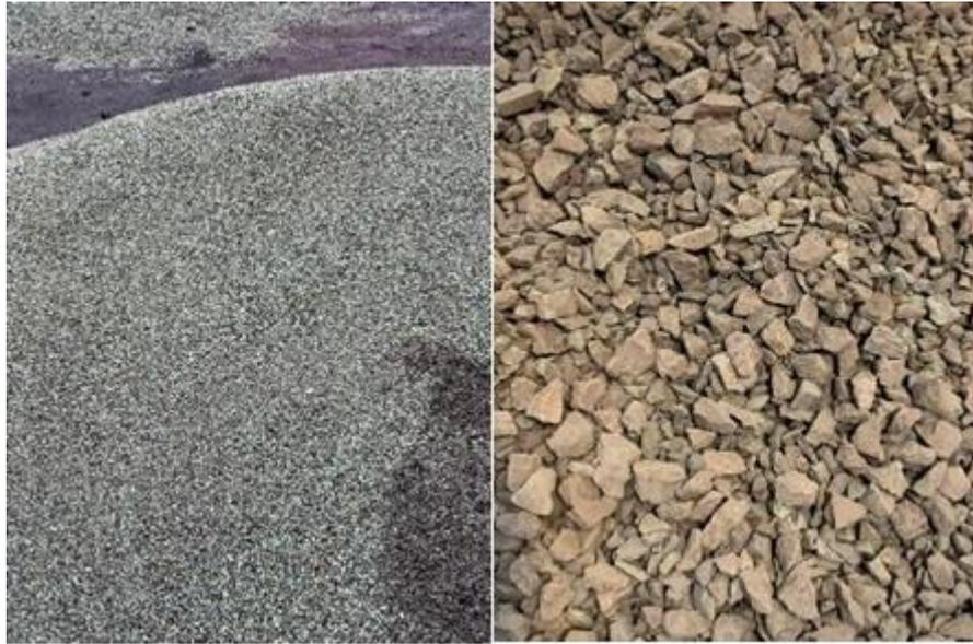
**Fig. 2.** Ferro-silicomanganese slag of ferroalloy industries.
