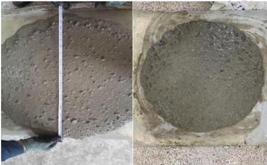
**Fig. 3.** SCC slump-flow test.
