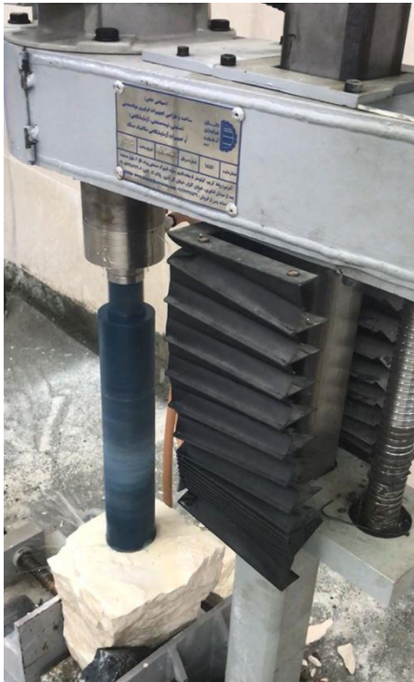
Fig. 5. Coring device while the core capturing.
