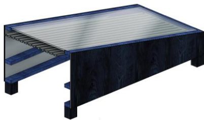
Figure 7. Designed Flat Plate Solar Collector
