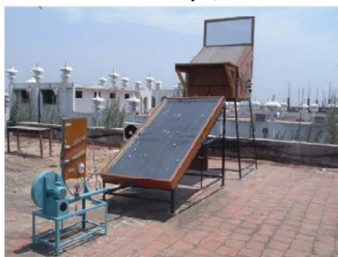
Figure 3: Pictorial view of the desiccant integrated solar dryer with reflected mirror [31]. (This is an example of an active solar dryer)
