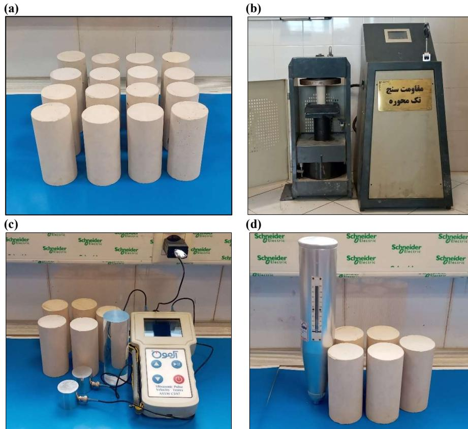
**Figure 2.** (a) Some specimens prepared for laboratory tests including (b) uniaxial compressive strength (UCS), (c) P-wave velocity ( $V_p$ ), and (d) Schmidt hardness (SH)
