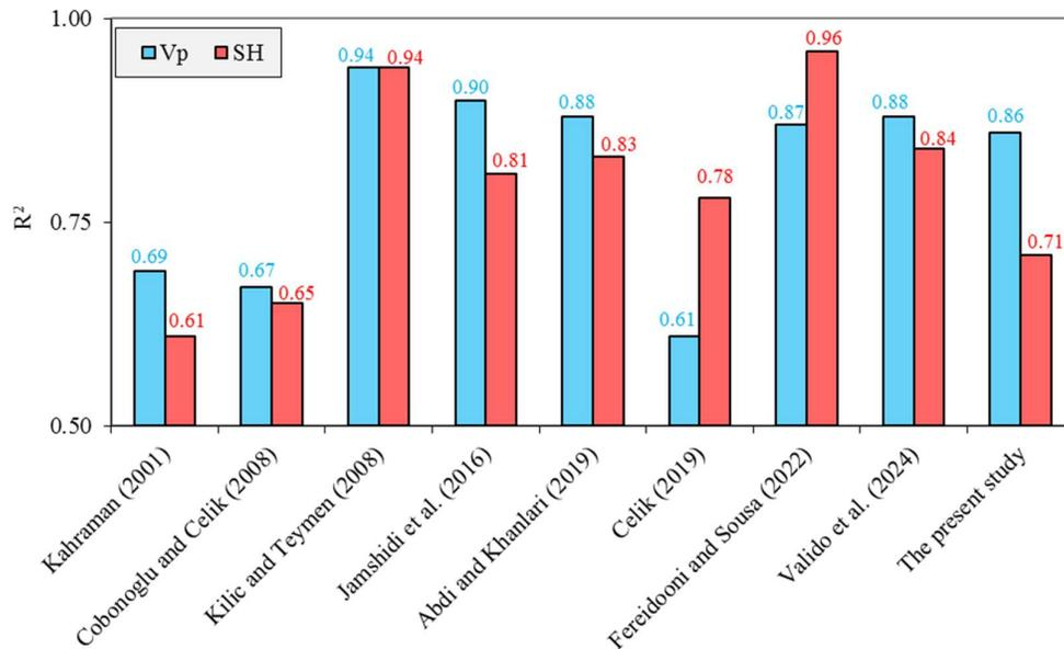
**Figure 7.** The  $R^2$  values of the correlation equations developed for predicting the UCS from Vp and SH
