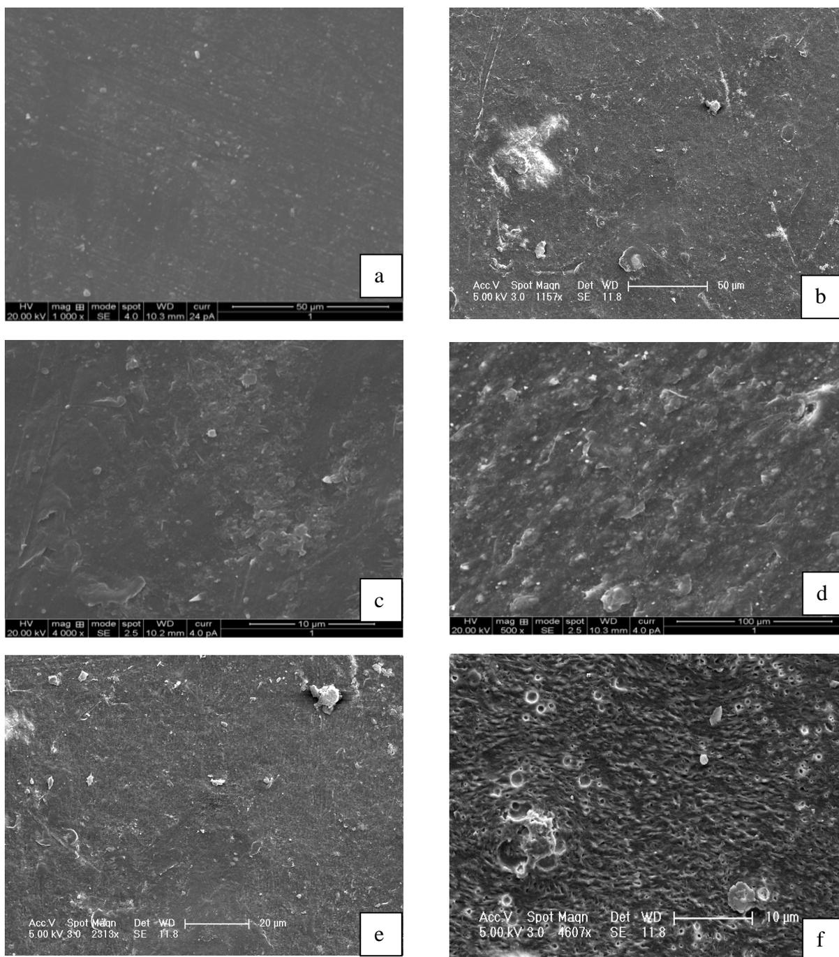
**Fig. 1. SEM photograph of (a) control polyethylene and polyethylene treated with (b) *Curvularia lunata* (c) *Alternaria alternata* (d) *Penicillium simplicissimum* (e) *Fusarium* sp. and (f) consortium**
