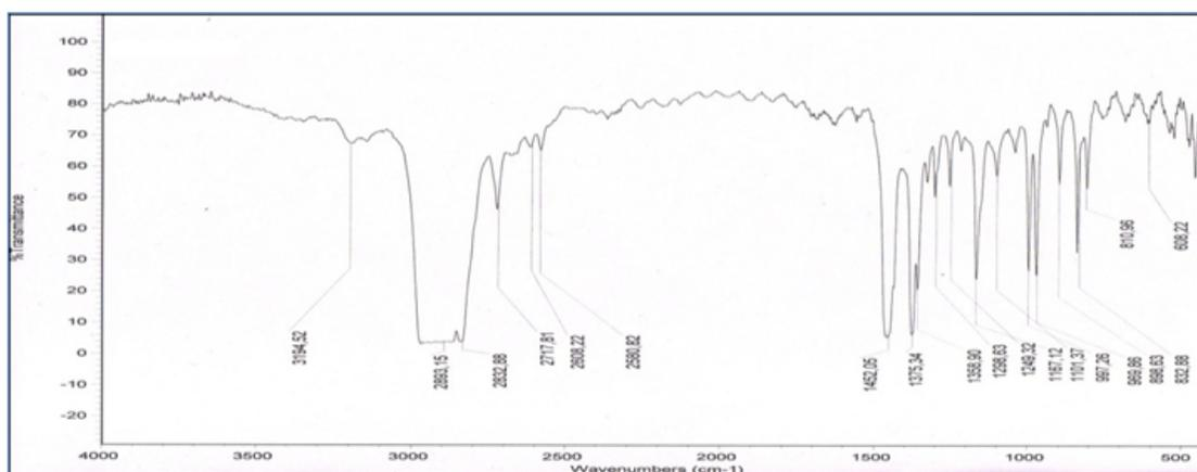
Fig.7. FTIR spectrum of polyethylene treated with consortium (*C. lunata*, *A. alternata*, *P. simplicissimum* and *Fusarium sp.*)
