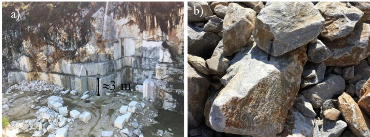
Figure 3. Sampling at a typical marble quarry in the investigated area; a) Chain saw cutting method, b) Collected bulk samples.
