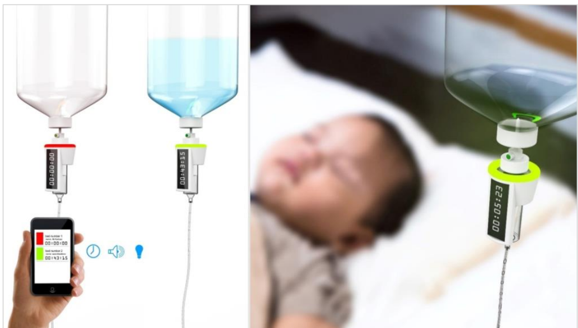
Figure 8: Conceptual design - Wireless monitoring and a mobile alarm system for nurses can offer parents peace of mind, minimize disruptions for nurses, and promote greater autonomy for children (Designed by the writer).
