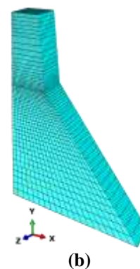
Fig. 7. Details of Koyna dam: a) Geometrical dimensions of the Koyna dam (Chopra and Chakrabarti, 1973); and b) FE mode of Koyna dam
