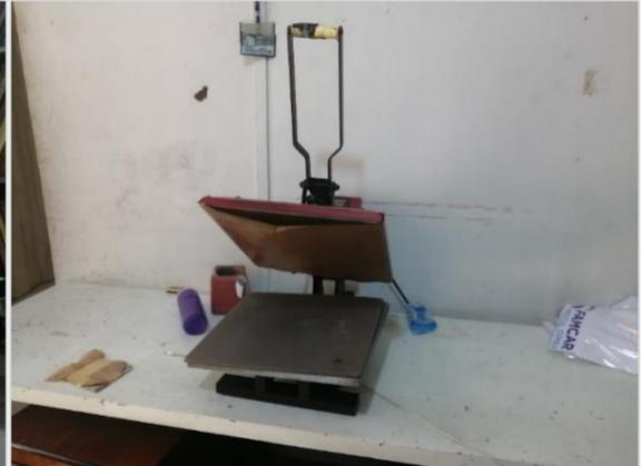
Figure 3: Heating Pressing Machine (Curing).
