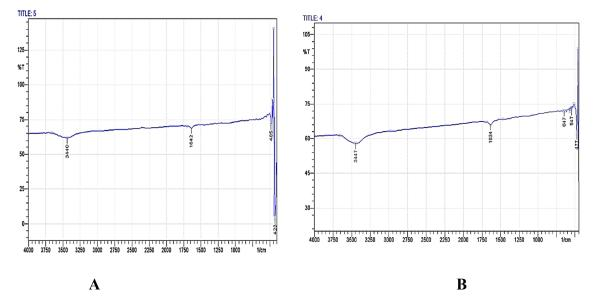
Fig. 4. A and B: FTIR infrared spectral tests (peaks spectra for microplastic compounds) in raw water for Al-Fahama station
