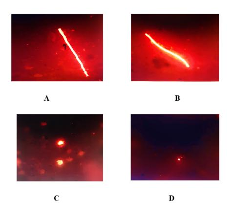
Fig. 3. Microscopic examination of microplastics by the fluorescent microscope (A, B) Fibre shape (C) Granules or Pellets shape, (D) Fragments
