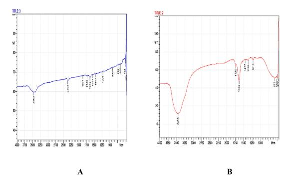
Fig. 5. FTIR infrared spectral tests (peaks spectra for microplastic compounds) (A) Drinking water and (B)Rraw water for AL- Fateh AL-Mubin station
