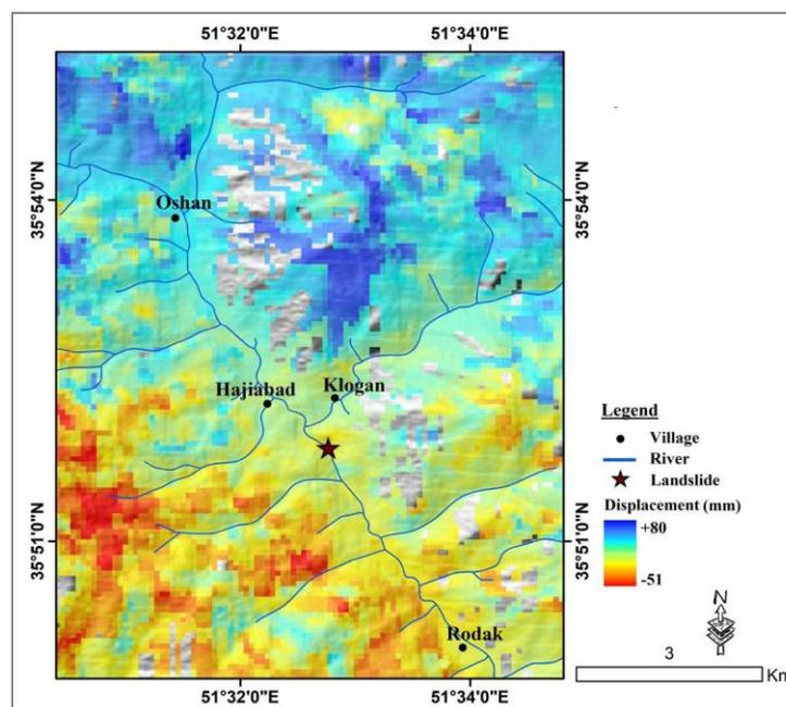
**Fig. 7.** The vertical displacement of the region from 01/06/2016 to 12/21/2018
