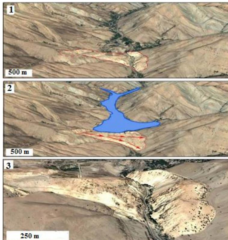
**Fig. 5.** 1) Cutting off the landslide dam and the drainage of the dam lake and remaining lake terraces. 2) Reconstruction of the dam lake at the time of the landslide and the formation of the landslide dam lake. 3) The landslide mass in the current conditions (Google Earth).
