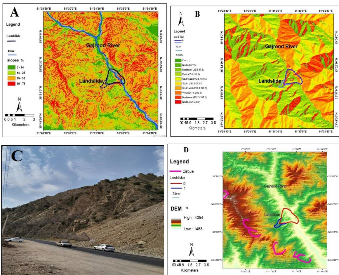
**Fig. 4.** A. slope, B Aspect Slope, C. Rudak fault zone (stratification disruption due to crossing the Rudak fault line), D. Position of dominant cirques upstream of the Jajrud landslide.
