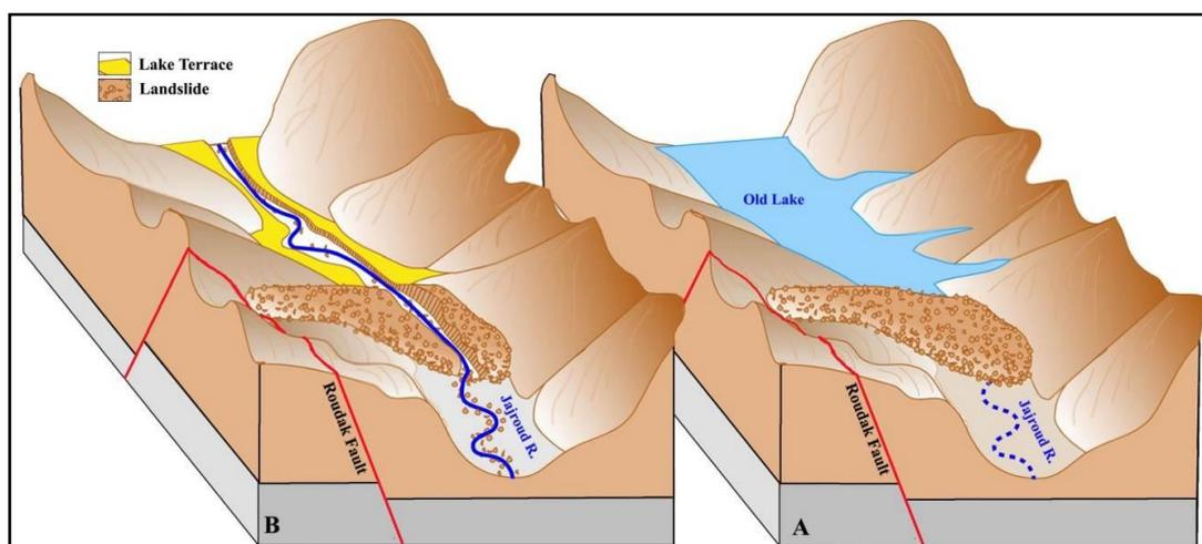
**Fig. 6.** Block diagram of the Jajrud Valley A. Reconstruction of the lake at the time of landslide and formation of the landslide Dam Lake B. Rupture of the landslide dam and remaining lake terraces as ancient legacies of lake formation.
