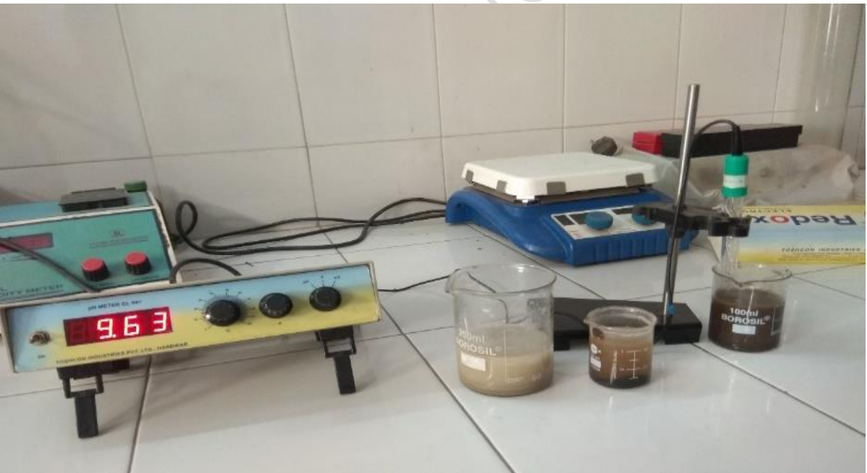
Fig. 5. Setup for the determination of pH value test
