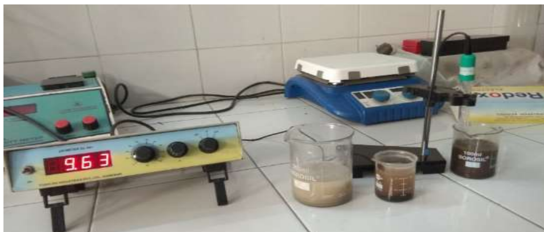
Fig. 5. Setup for the determination of pH value test
