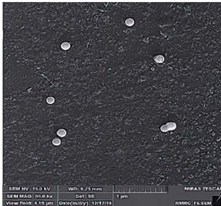
Fig 1. SEM image of selenium nanoparticles, with an average size of about 200 nm. DLS analysis revealed 206 nm nanoparticle size and a 0.231 particle size distribution, indicating particle size uniformity (Figure 2).
