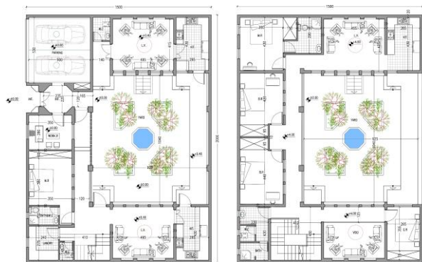
Figure 5. documents and proposed plans of the second option (traditional architecture of the region); Left to right: ground-floor plan, first-floor plan
