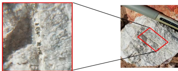
Figure 16. View of a veinlet with mineralization of pyrite, chalcopyrite, and molybdenite in hand sample.
