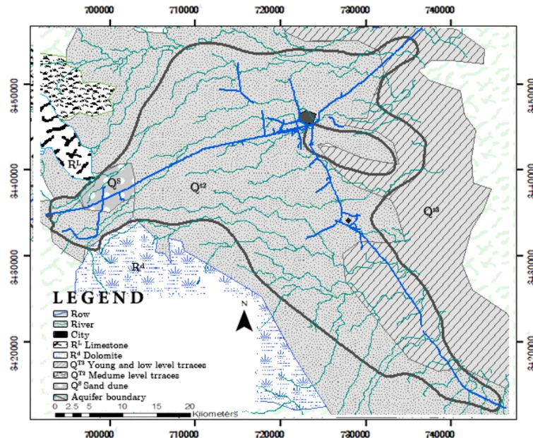
**Figure 1.** Geological map of the Abarkooh plain in which Iso-potential lines and groundwater flow directions are also depicted
