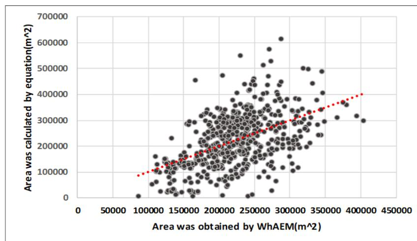
**Figure 6.** The correlation between the capture zone area calculated by WhAEM and multi-variate regression
