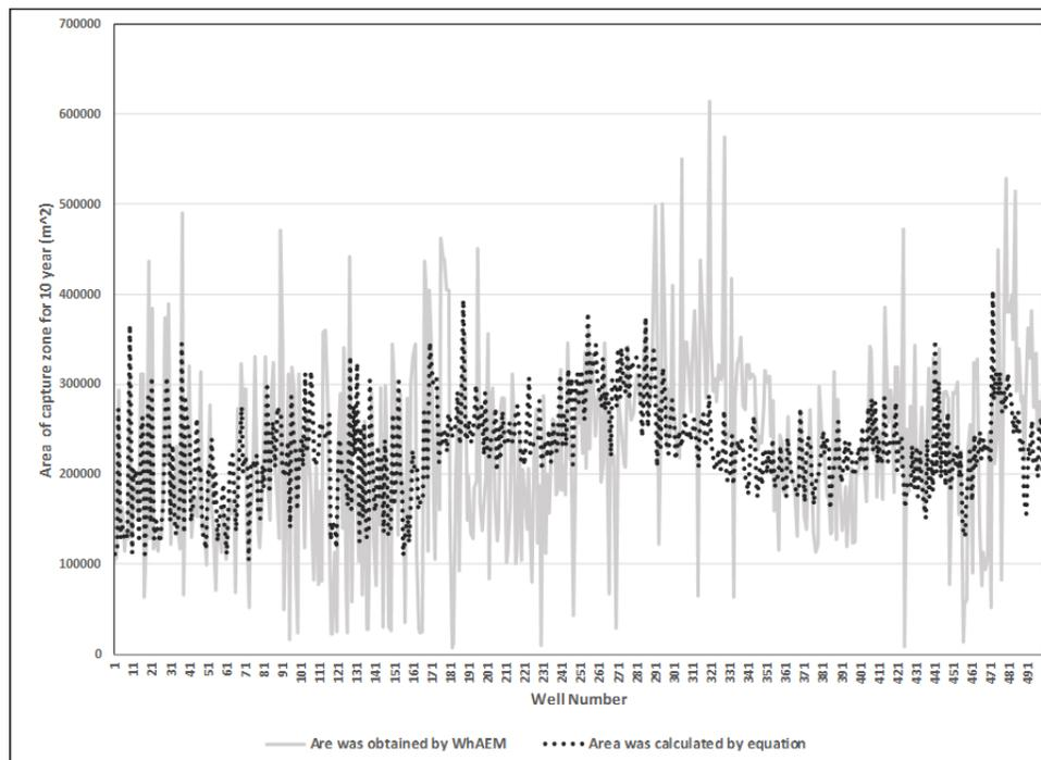
**Figure 5.** Comparing the area of the capture zone calculated by the WhAEM software and proposed equation derived by multivariate regression method
