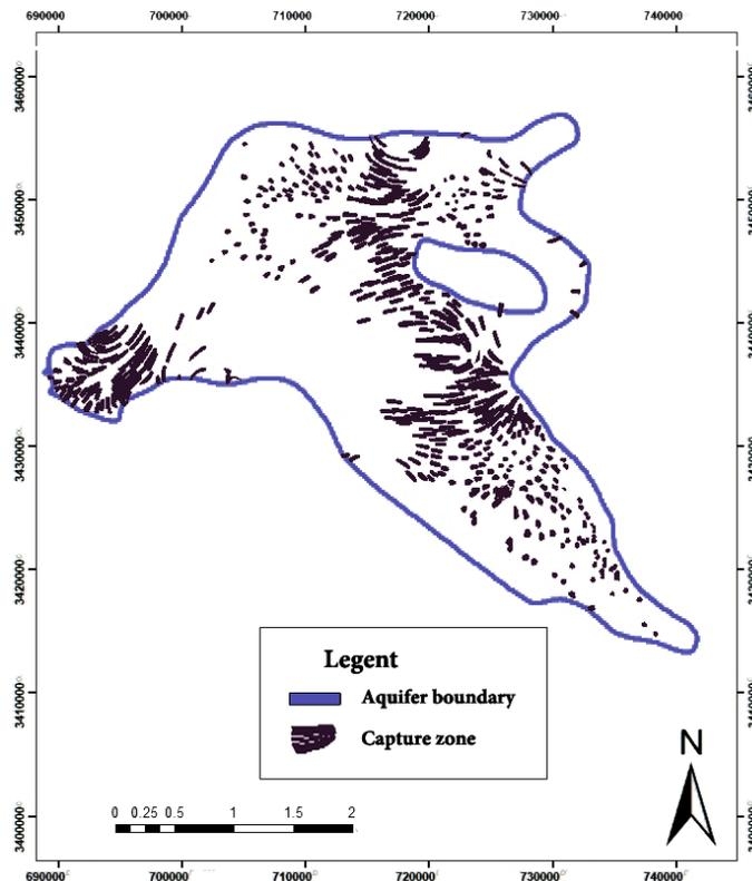
**Figure 4.** The capture zone of the production wells in Abarkooh aquifer based on the results of the WhaEM calibrated model
