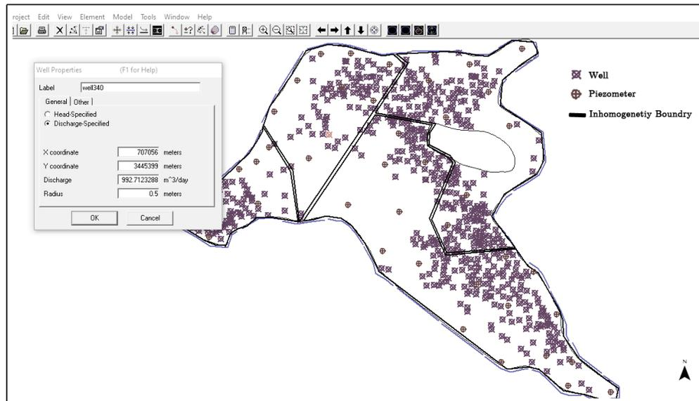
**Figure 3.** The WhaEM model for the estimating capture zone of the wells in the study area
