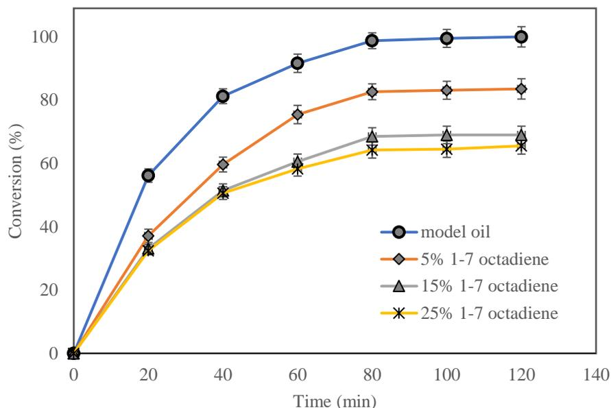
Fig. 5. The impact of 1-7 octadiene on ODS mixed model oil
