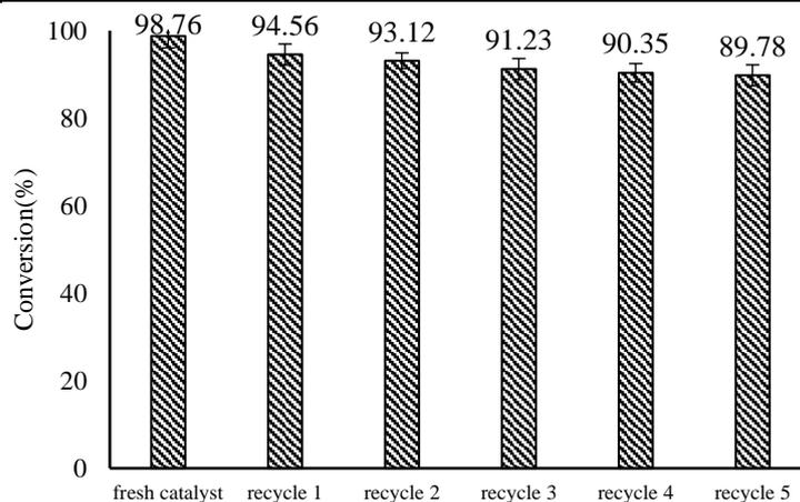
Fig. 1. Influence of the recycle times on ODS of mixed model oil
