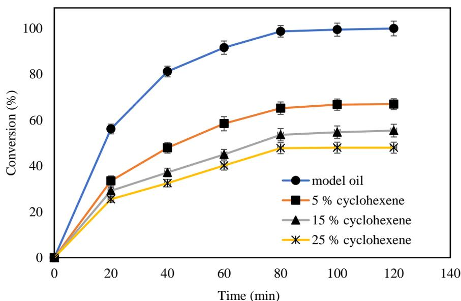
Fig. 4. The impact of cyclohexene on ODS mixed model oil
