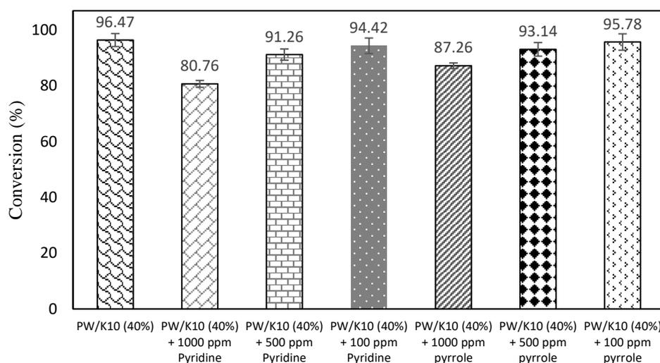
Fig. 6. The effects of pyridine and pyrrole on ODS 1000 ppm mixed model oil and MeCN
