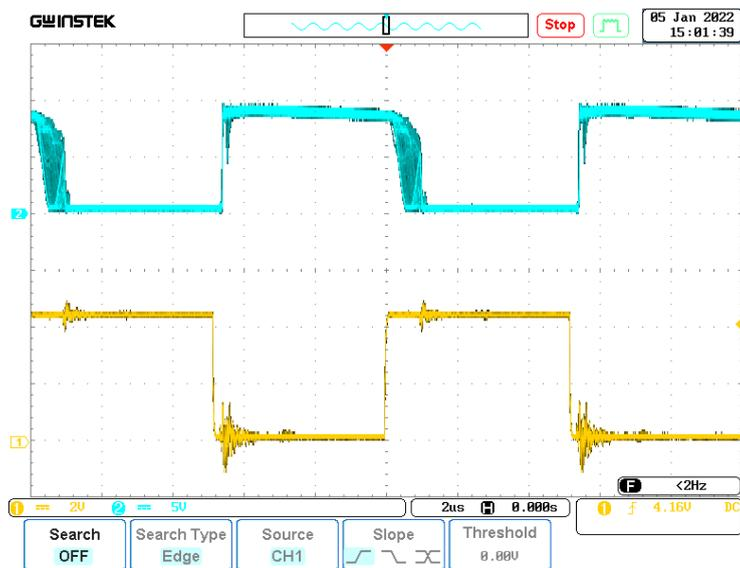
(a) The diode' voltage  $D_{forward}$
