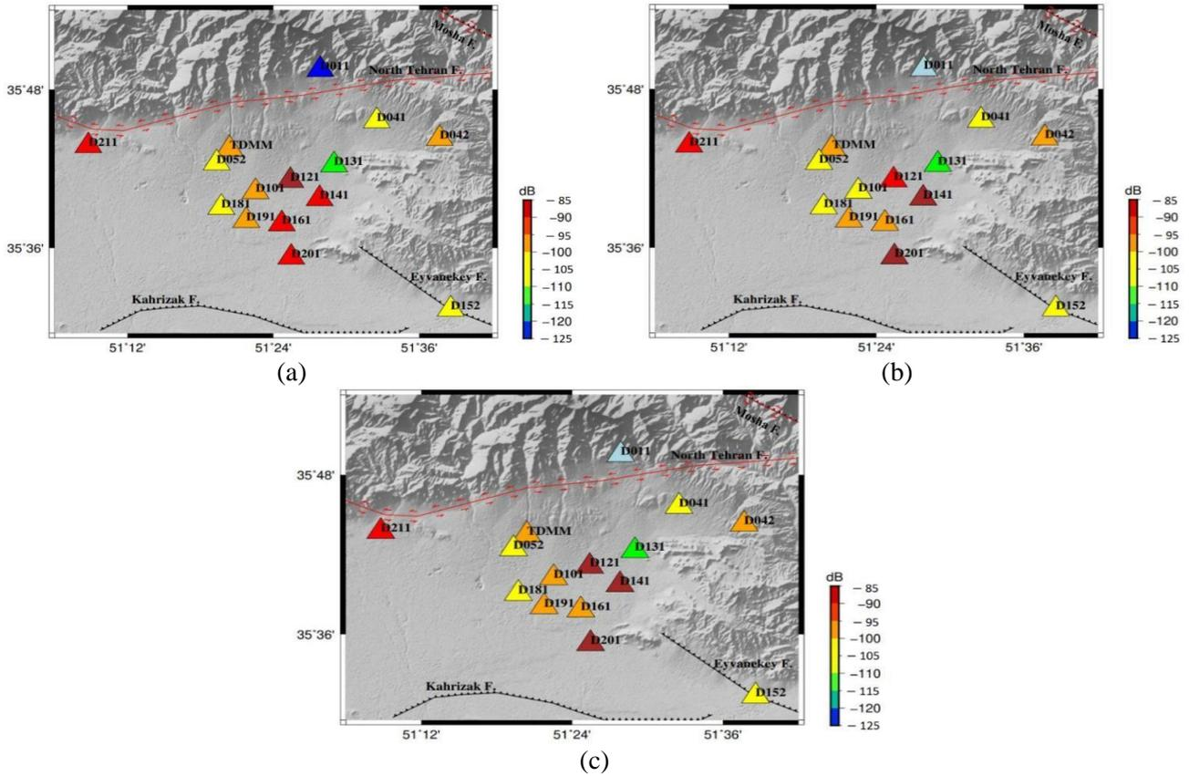
Figure 3. Spatial variations of the lowest median of the PDF related to the frequency range 8-12 Hz for a) Z-component, b) N-component, c) E-component.
