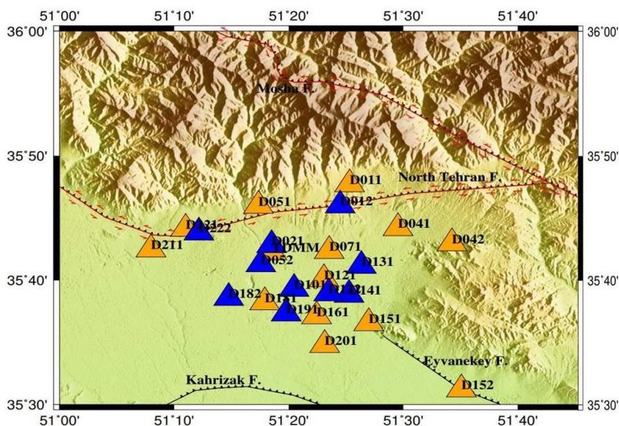
**Figure 1.** The accelerometer stations used in this research. The orange triangles show the accelerometer stations of the TDMMO network, and the blue triangles are the accelerometer stations of the BHRC, which are joint with the TDMMO. Red lines indicate faults with a strike-slip mechanism, and black lines indicate faults with a reverse mechanism.
