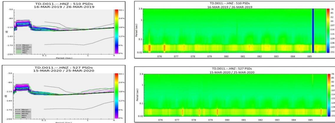
**Figure 5.** An example of PSD-PDF map obtained from PQLX software for the Z-component of D011station in the frequency domain.
