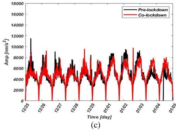
**Figure 8.** Envelope of accelerometer filtered between 8 and 12 Hz for pre-lockdown and co-lockdown for components (a) Z, (b) N and (c) E. Black line indicates the pre-lockdown and red line indicates the co-lockdown.
