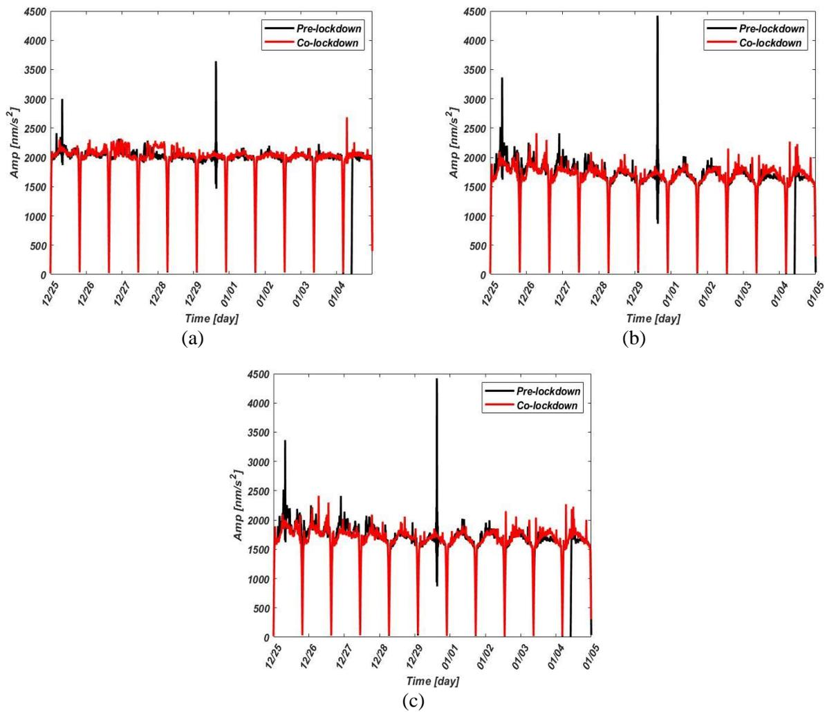
**Figure 7.** Envelope of accelerometer filtered between 2 and 6 Hz for pre-lockdown and co-lockdown for components (a) Z, (b) N and (c) E. Black line indicates the pre-lockdown and red line indicates the co-lockdown.
