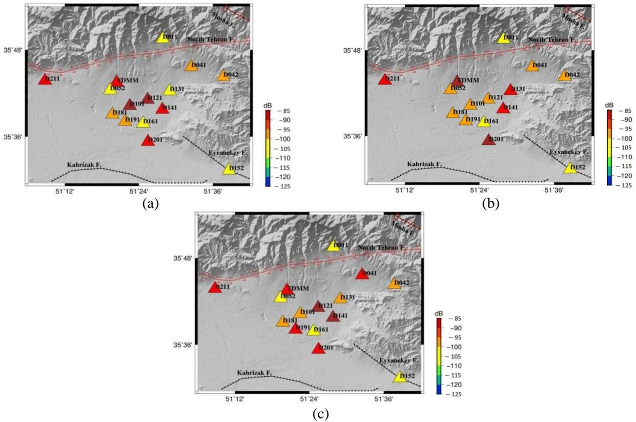
Figure 4. Spatial variations of the lowest median of the p PDF related to the frequency range 20-30 Hz for a) Z-component, b) N-component, c) E-component.
