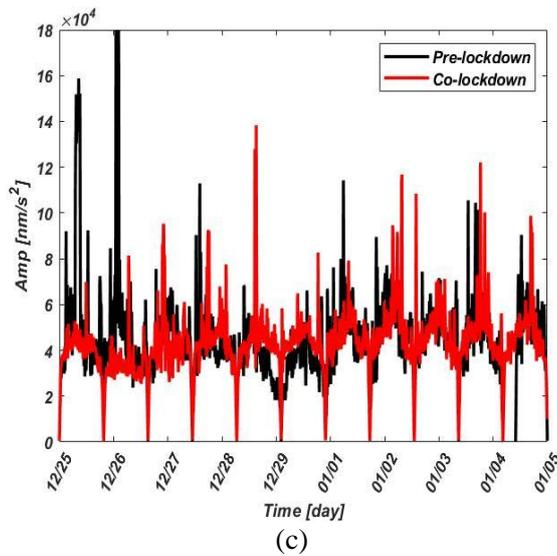
**Figure 9.** Envelope of accelerometer filtered between 20 and 30 Hz for pre-lockdown and co-lockdown for components (a) Z, (b) N and (c) E. Black line indicates the pre-lockdown and red line indicates the co-lockdown.
