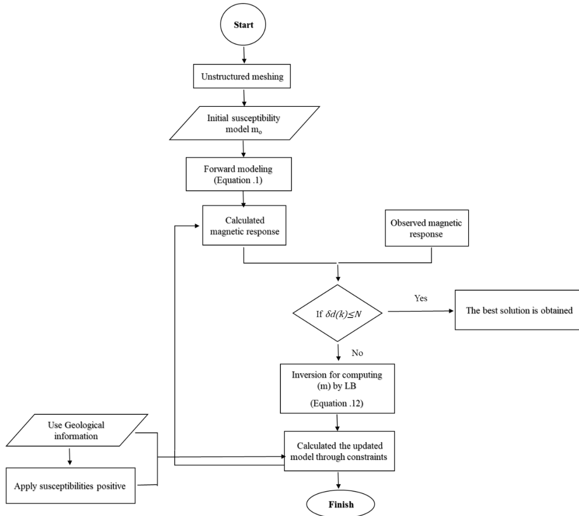
Figure 2. Workflow for inversion the proposed algorithm on magnetic data.
