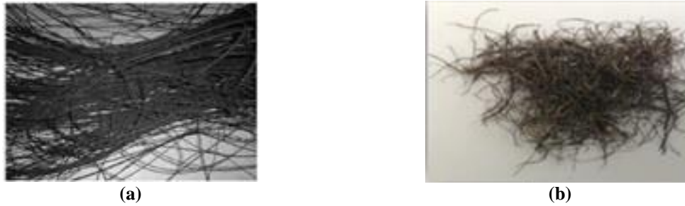
Fig. 2. The recycled fibers from: a) The thermal (Tlemat et al., 2003); and b) Cryogenic (Zamanzadeh et al., 2015) methods
