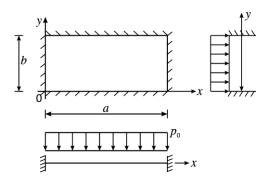
Figure 1: Clamped plate subjected to uniformly distributed load intensity  $p_0$
