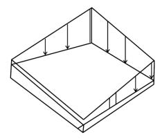
Figure 3: Hydrostatically loaded thin clamped rectangular plate
