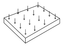
Figure 2: Uniformly loaded thin plate with clamped edges
