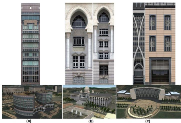
Figure 19. Producing textures via symmetrical left-right transformation (a) is Putrajaya Holding department, (b) is the Court of Justice and (c) is the Ministry of Finance.
