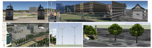
Figure 22. 3D models of statues, annexes between the departments, fences and lampposts based on Alpha channel.
