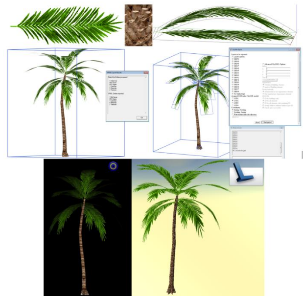
Figure 23. Illustration of designing a palm tree and converting it from SKP to VRML (BitManagement) and CityGML (LandXplorer) including 892 faces, 653edges, and 2 texture files.
