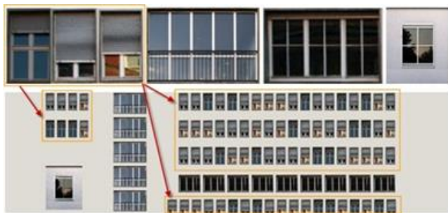
Figure 3. One pixel is used for the wall texture and three random textures are used for three window layers to increase the Level of realism.
