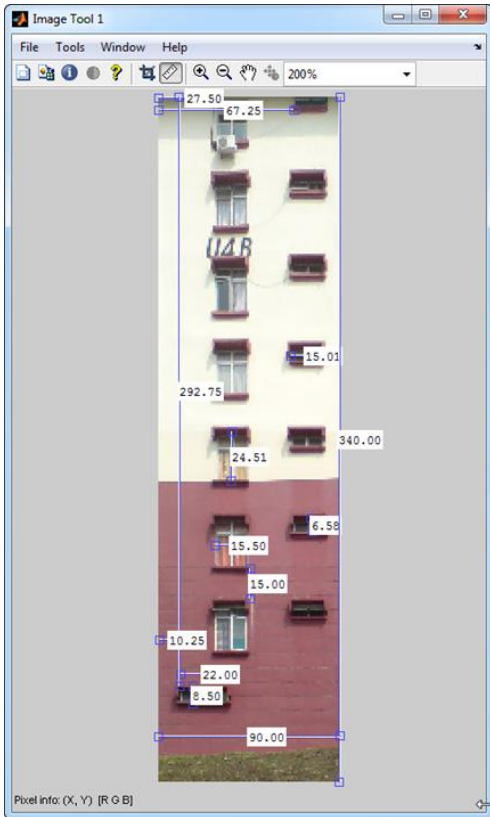
Figure 6. Measuring all the required parameters for DPF via programming in Matlab in pixel unit.
