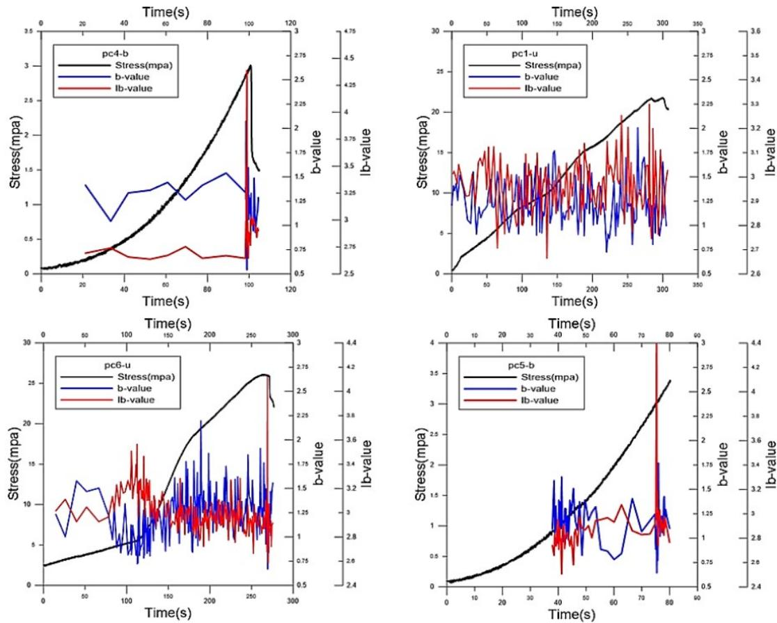
**Figure 13.** Chart of the changes in b-value and Ib-value and the loading stress for uniaxial (pc6-u, pc1-u) and tensile splitting (pc5-b, pc4-b) tests
