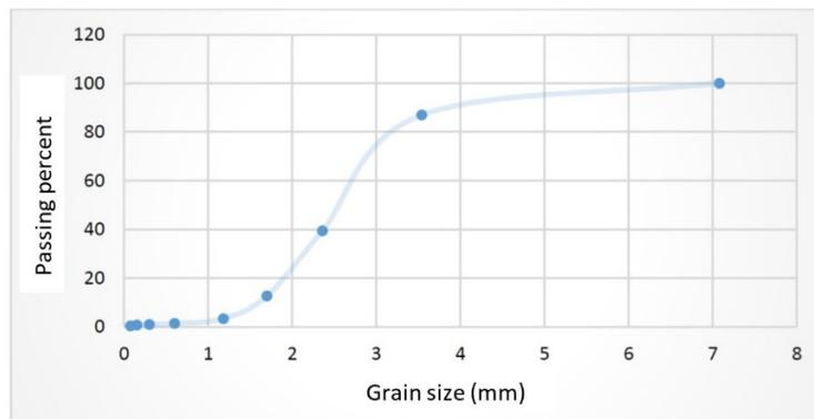
**Figure 1.** Particle Size Distribution of aggregate by Sieve Analysis
