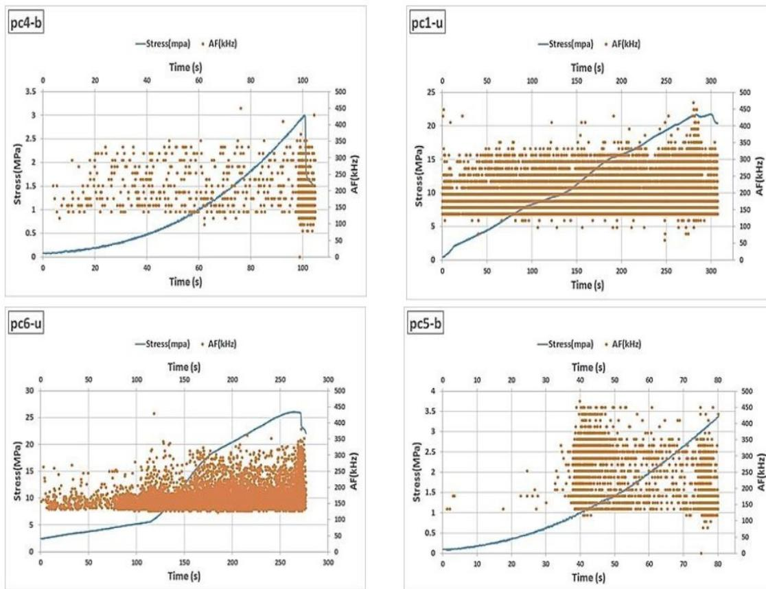
Figure 7. Chart of average frequency changes and loading stress in tensile splitting (pc5-b, pc4-b) and uniaxial (pc6-u, pc1-u) tests
