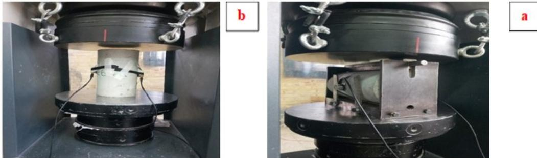
**Figure 2.** testing procedure, (a) tensile splitting test, (b) uniaxial compressive strength test
