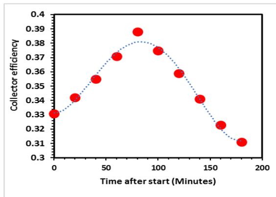
Figure 5 Collector’s efficiency changes during the test.
