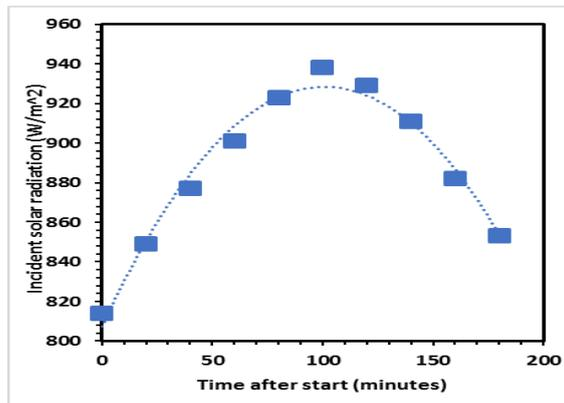
Figure 3 Solar radiation reaching the collector during the experiment
