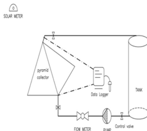
Figure 1 Schematic of equipment placement for experimental measurement of collector efficiency.
