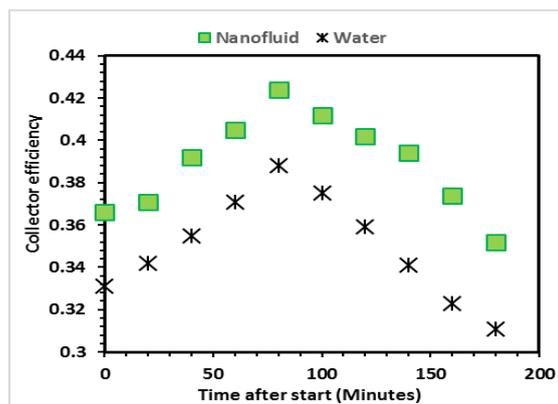
Figure 9 Effect of copper-water oxide nanofluid and ordinary water on collector efficiency.
