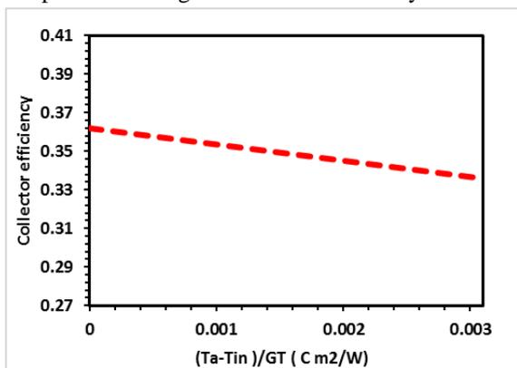
Figure 7 Evaluation of collector efficiency based on temperature reduction criteria.
