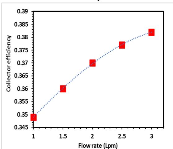
Figure 10 Investigation of the effect of volume flow on collector efficiency.
