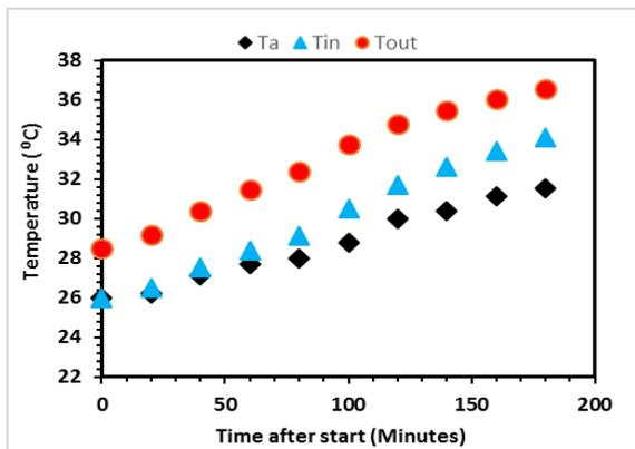
Figure 6 Changes an inlet, outlet, and ambient temperature during the collector efficiency test.
