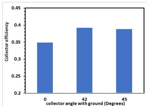
Figure 11 Investigating the effect of collector installation angle on efficiency.
