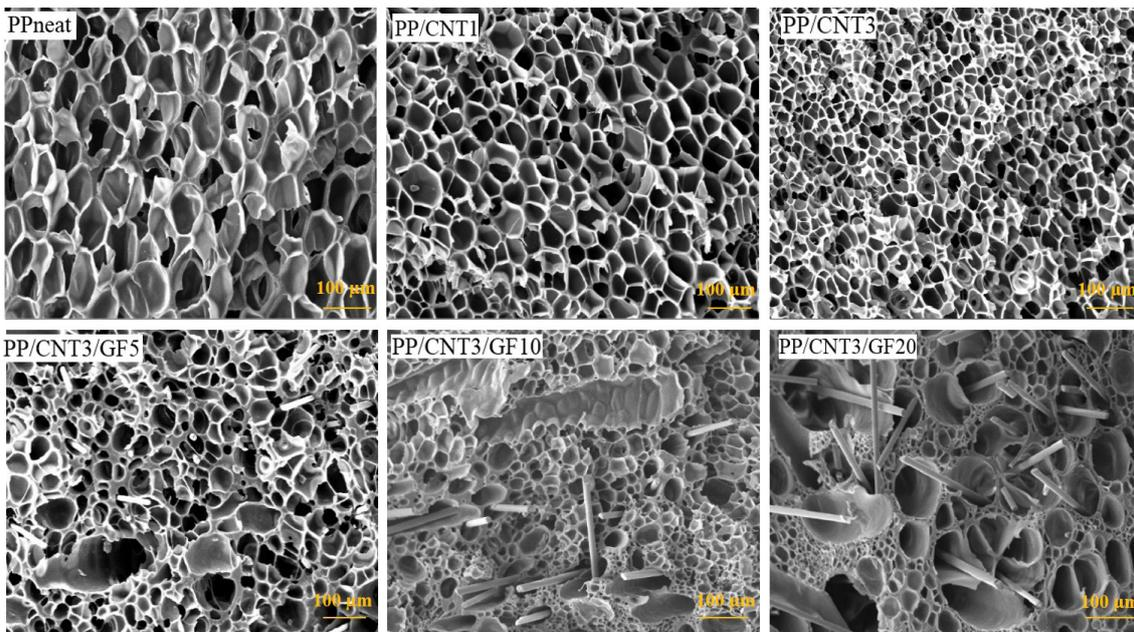
Fig. 2- SEM micrographs and cell size distribution of the produced foams.
