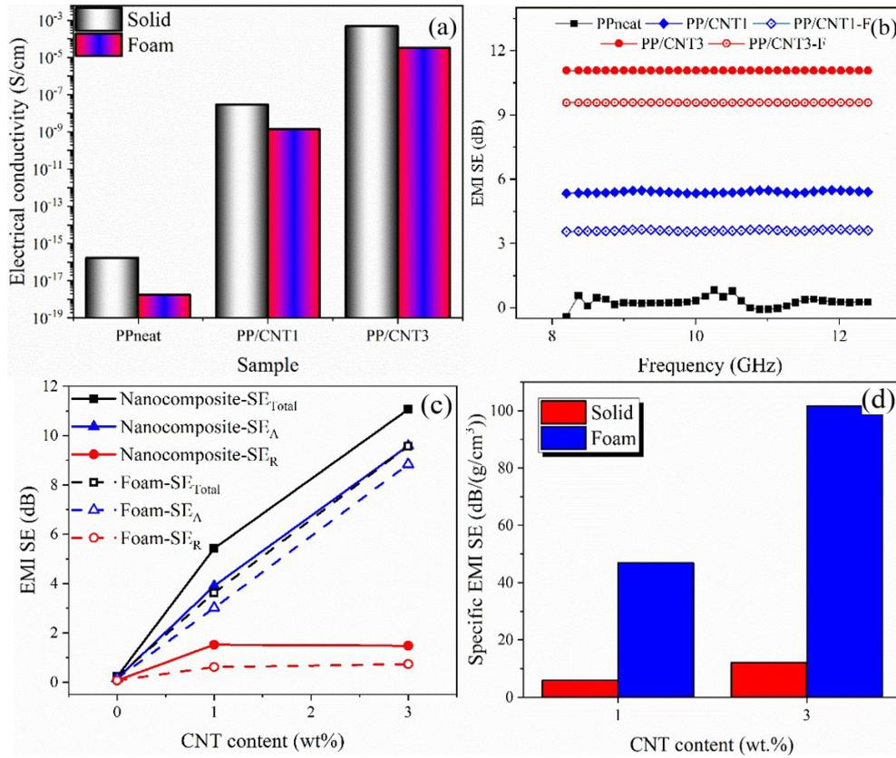
Fig. 3- (a) Electrical conductivity (b) EMI shielding efficiency (c) SETotal, SER, and SEA of nanocomposites and foams (d) Specific EMI shielding efficiency.
