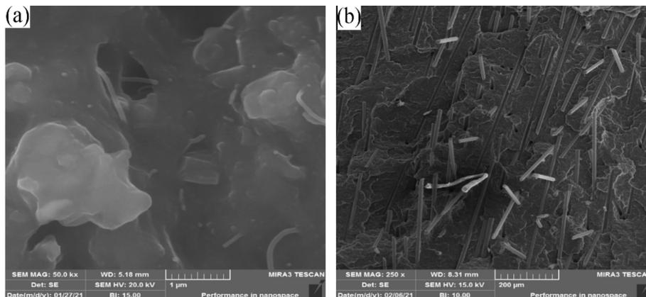
Fig. 1- FE-SEM images of cryo-fractured surfaces of PP/CNT3 and PP/CNT3/GF10.
