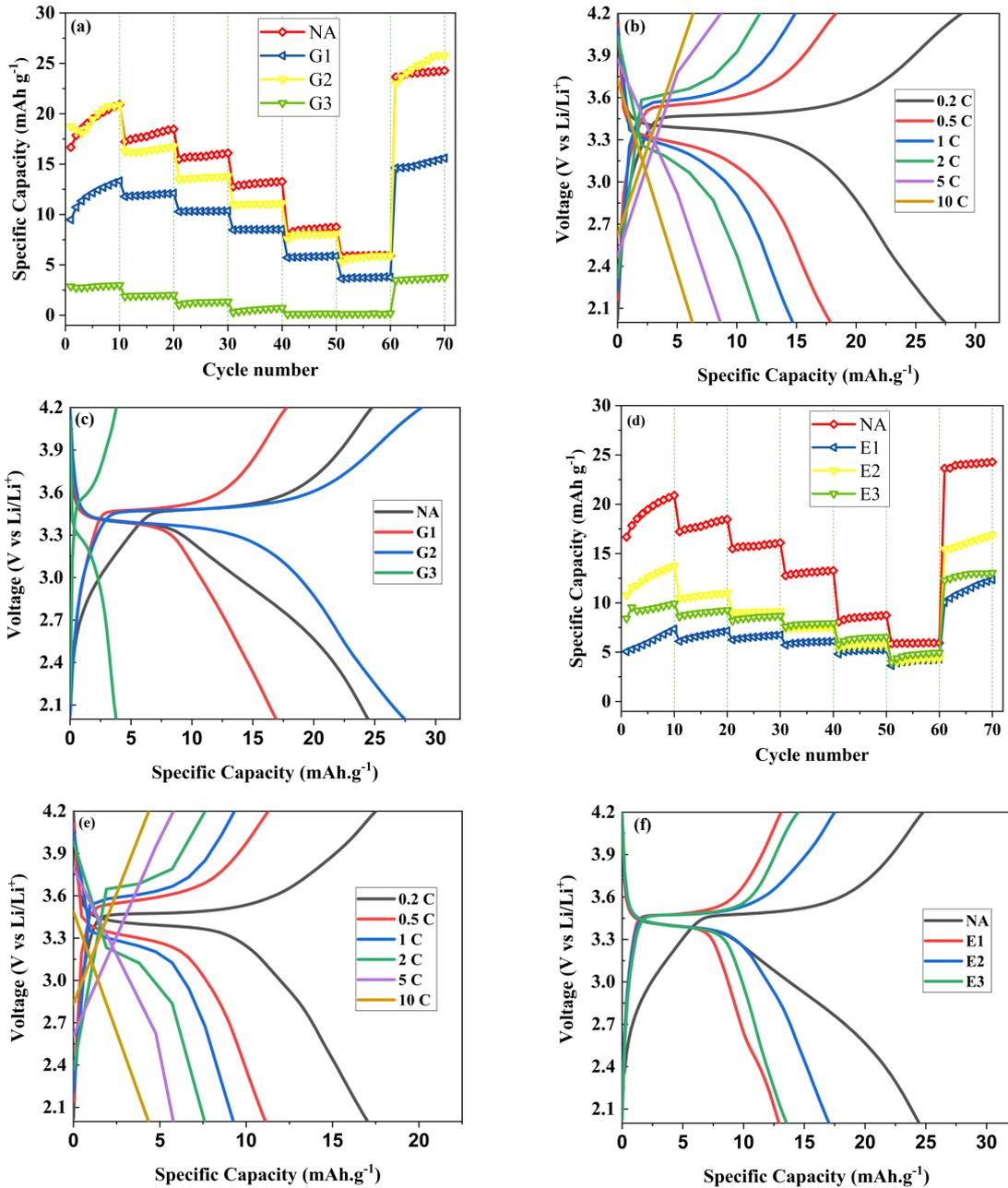
Fig. 6- Results of specific capacity obtained from (a) glycine and (d) l-glutamic acid at different charge and discharge rates, charge / discharge curves at different rates for (b) G2 and (e) E2 samples which had the highest capacity, and the comparison of charge and discharge curves of the (c) glycine and (f) l-glutamic acid samples with no amino acid sample at 0.2C rate.
