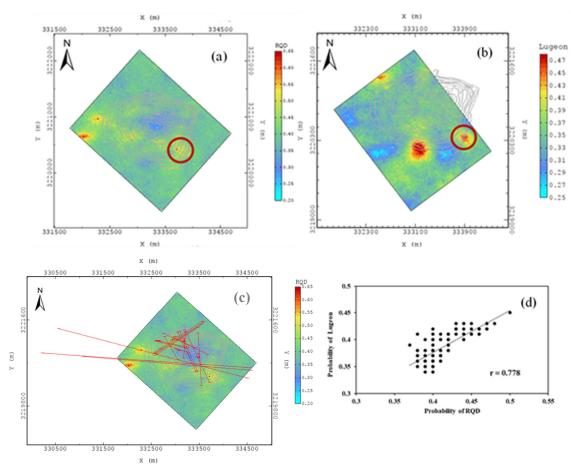
**Figure 9.** Map of the mean probability of RQD less than 30 (a) and Lugeon greater than 2 (b) correlation between the mean probability of the RQD and Lugeon in the southeastern of the pit (c) and matching of the faults on the map of the mean probability of RQD less than 30 for final level of the pit to boundary between the dense alluvium layer (d).
