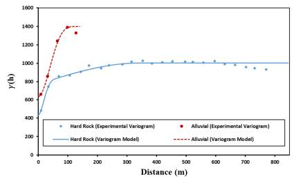
**Figure 3.** Comparison experimental variograms (points) and fitted variogram model (lines) for the dense alluvium and hard rock formation
