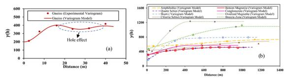
**Figure 6.** The RQD experimental variograms and fitted variogram model for (a) Gneiss lithology and (b) lithology of Amphibolites, Bottom Magnetite, Quartz Schist, Conglomerate, Skarn, Oxidized Magnetite, Bressia zones and Chloritic Schist
