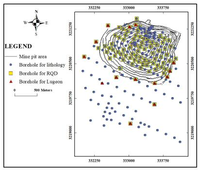
Figure 2. The location of various boreholes inside and outside of the Gohar-Zamin mine pit
