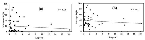
Figure 5. Correlation between minimum values (a) and average values (b) of RQD with Lugeon
