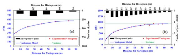
**Figure 7.** The RQD experimental variograms and fitted variogram model for various height levels, (a) 1150-1250 m, (b) 1550-1650 m
