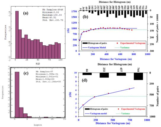
Figure 4. Histogram and omnidirectional variograms for RQD (a and b) and for Lugeon (c and d)
