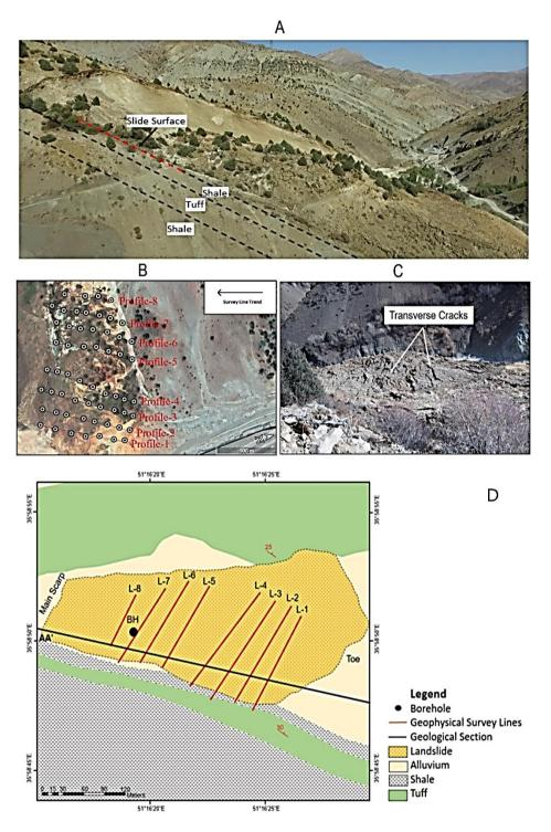
Fig. 4. (a) 3D view of the sliding surface. (b) plan view of data acquisition points. (c) An image of the transverse cracks near the toe of the landslide. (d) Geoelectrical profiles and location of the borehole [25].
