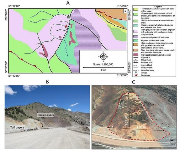
Fig. 3. (a) The research area's geological map. The major tectonic characteristics of the area are also depicted. (b) Presence of alternative tuff and shale layers in the vicinity of landslide area [25], (c) landslide body with its dimensions measured about 170 m in width and extends down to slope in the length of about 357 m.
