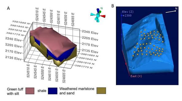
Fig. 9. 3D view of (a) geological map, and (b) location of 58 electrodes.
