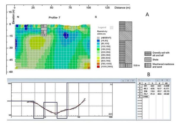
Fig. 6. (a) Inversion model of profile 7 accompanied by drilling borehole, (b) the sounding curve of the closest point to the borehole using IPI2WIN software.
