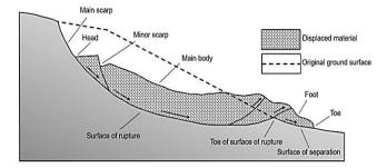
Fig. 1. A simple illustration of a landslide (reproduced from the work by Highland and Bobrowsky, 2008) [31].
