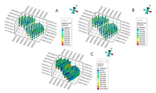
Fig. 5. 3D view of (a) observed apparent resistivity, (b) calculated data, and (c) inverted model.
