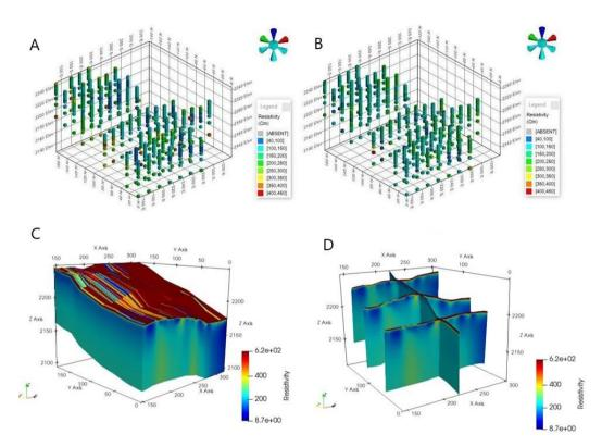
Fig. 8. (a) observed resistivity model, (b) calculated resistivity model, (c) 3D inverted resistivity image model, (d) 3D resistivity contour plot.
