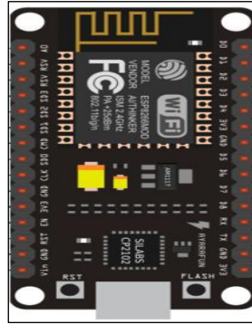
Figure 6. Circuit Diagram of ESP8266 Wi-Fi Module or Unit.
