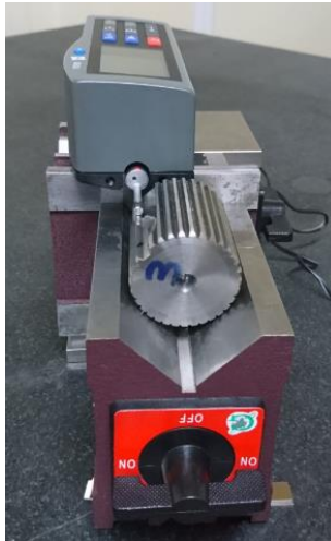
Figure 7: Measurement of surface roughness on the side surface of a spline tooth.
