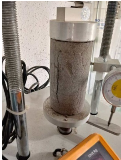
Figure 7. Uniaxial compressive strength (UCS) test on treated specimens
