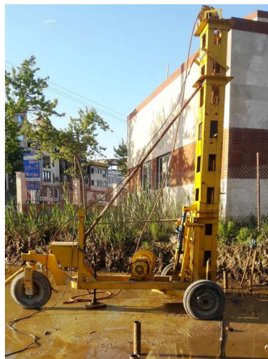
Figure 13. A typical hydraulic pipe-percussion machine used for micropiling in Iran
