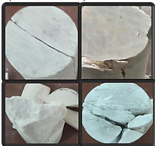
Fig5. Thermal breakage of Ghulmet marble specimens
