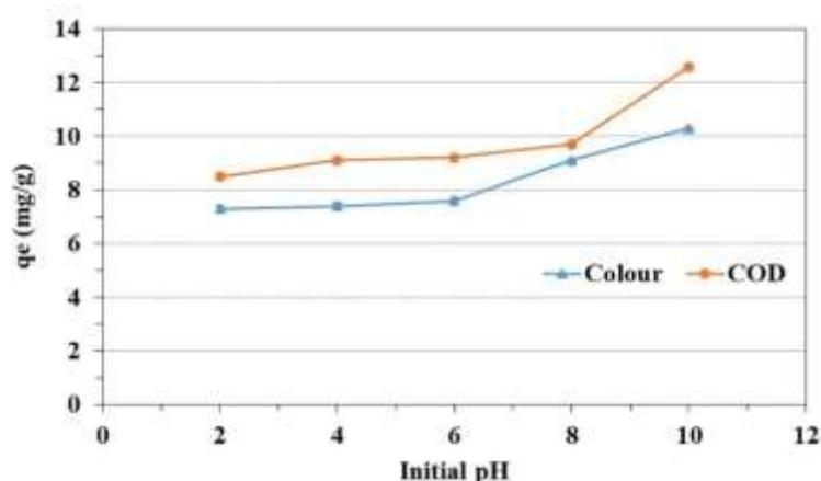
Fig. 10. The effect of the initial pH on the adsorption capacity
