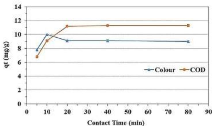
Fig. 8. The effect of the contact time on the adsorption capacity
