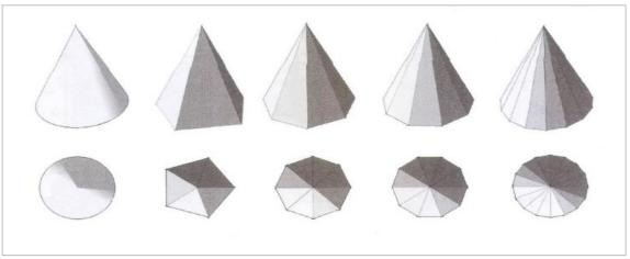
Figure 1: Various Shapes of Conical Dome (Memarian, 2013).
