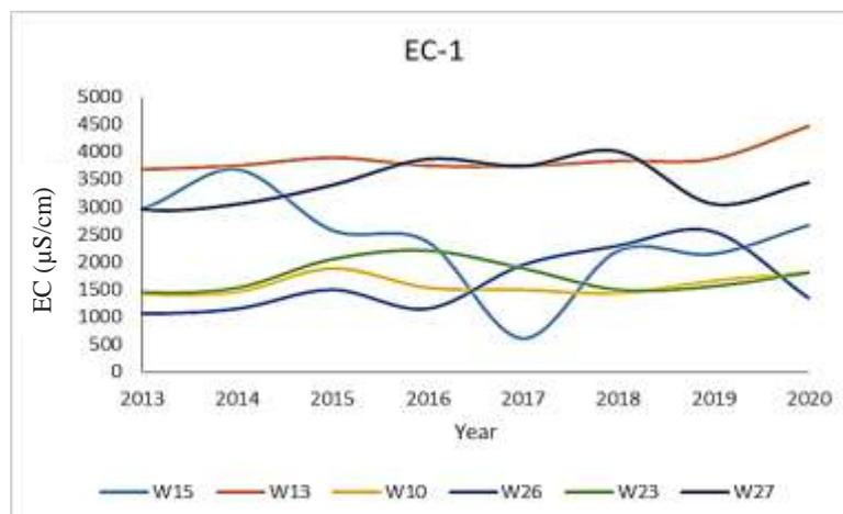
Fig. 4. Changes in the electrical conductivity of water ( $617 \leq EC \leq 5590$ )
