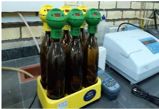
Fig 2B. Device for measuring BOD
