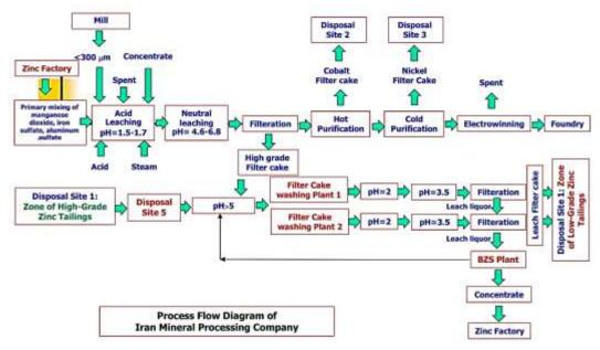
Fig 2. Zinc processing flow diagram in Iran Mineral Processing Company (IMPC)
