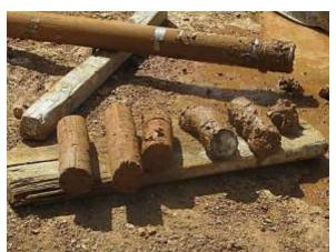
Fig 5. Undisturbed samples extracted by Shelby sampler during BH borehole drilling
