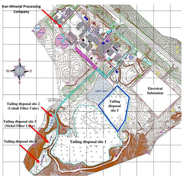
Fig 3. Site plan of Iran Minerals Processing Company and location of tailings disposal Sites 1 to 5
