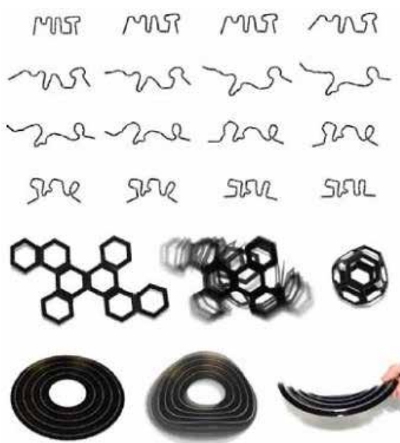
Fig. 8 A single strand that self-transforms from the letters “MIT” into the letters “SAL”(self-assembly lab), a flat surface that self-folds into a truncated octahedron, and a flat disc that self-folds into a curved-crease origami saddle structure
