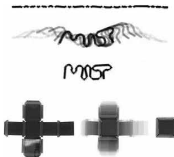
Fig. 7 A single strand that self-folds into the letters “MIT” and a flat surface that self-folds into a closed cube
