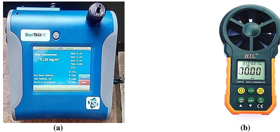
Figure.2: (a) Aerosol monitor DUSTTRAK™ (model 8530, TSI Inc. Mn) (b) Digital Anemometer Device AVM 06
