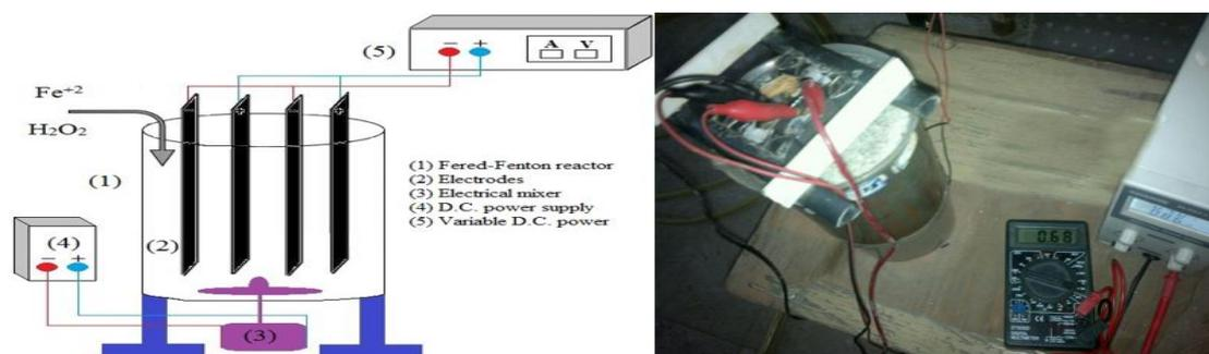
Fig. 1. Schematic and the picture of the Fered-Fenton reactor
