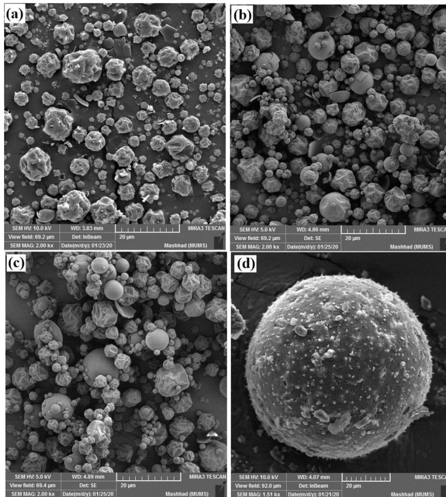
Fig.1. SEM image of saffron pollen capsule powder prepared at 140 °C (a) 160 °C (b), 180 °C (c) and non-capsule (d) (SEM magnification 2.00 kx).
