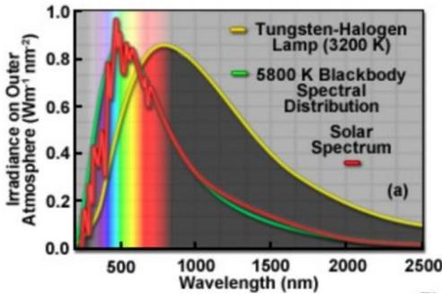
Figure 2 Tungsten Halogen lamp spectral distribution
