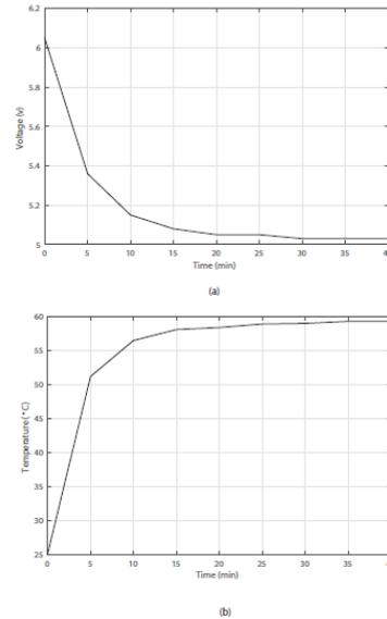
Figure 6. panel with no filter a) open loop voltage, b) surface temperature
