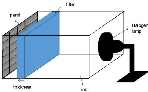
Figure 5. graphical view of the test setup
