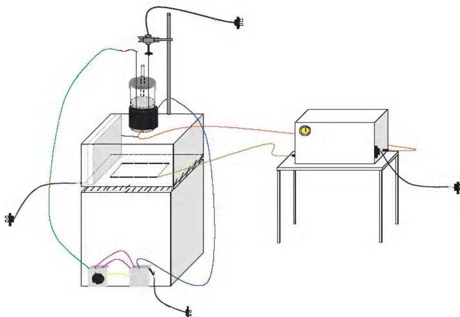
**Fig. 1. schematic diagram describing the melt-electrospinning technique**
