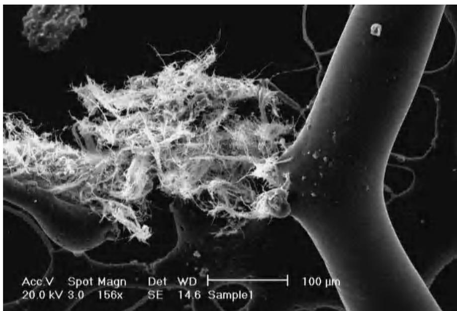
**Fig. 3. The SEM micrograph of morphology and diameter of PET fibers at electric field strength of 20 kV/cm and 9 cm distance between nozzle and collector**
