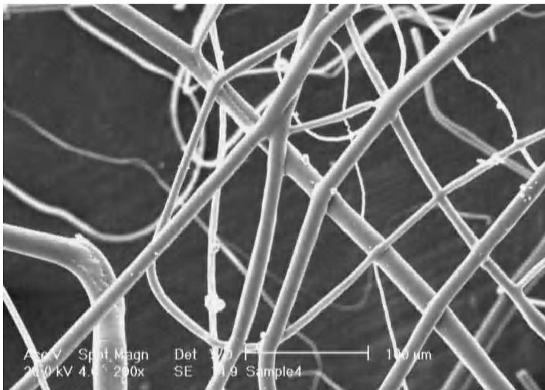
**Fig. 5. SEM photo micrograph for significant Effect of Processing Temperature on Fiber Diameter**
