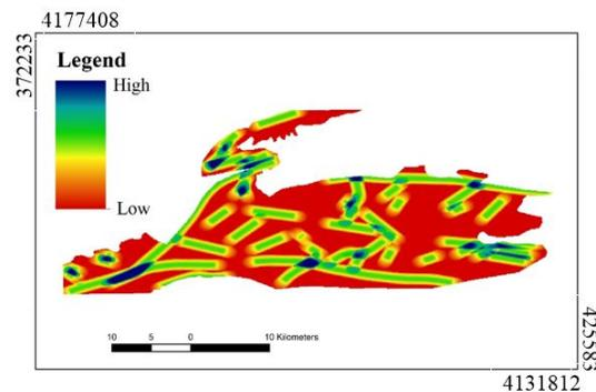
**Figure 5.** Fracture (lineament) density map of the Kalaleh basin
