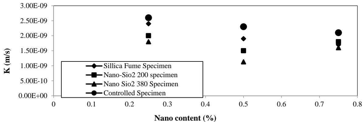
Fig. 13. Permeability of soil-cement mixtures with different silica materials
