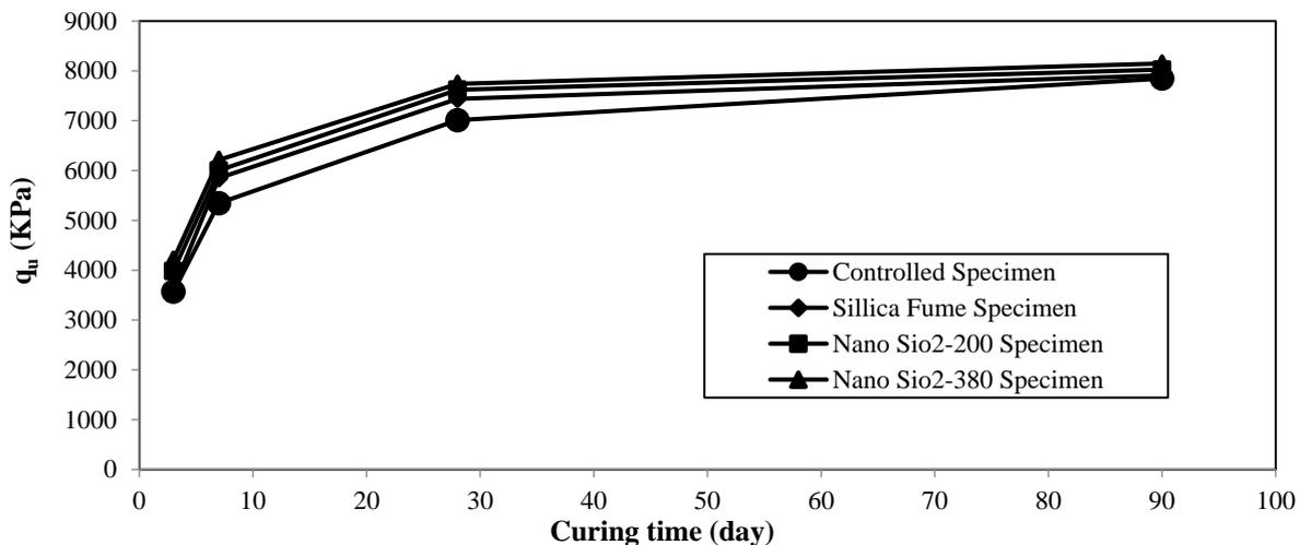
Fig. 10. Strength gain of soil-cement mixtures
