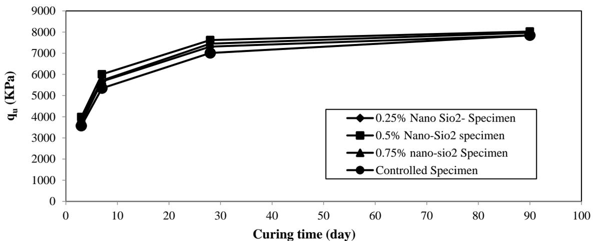
Fig. 11. Strength gain of the mixtures containing different percentages of nanosilica 200
