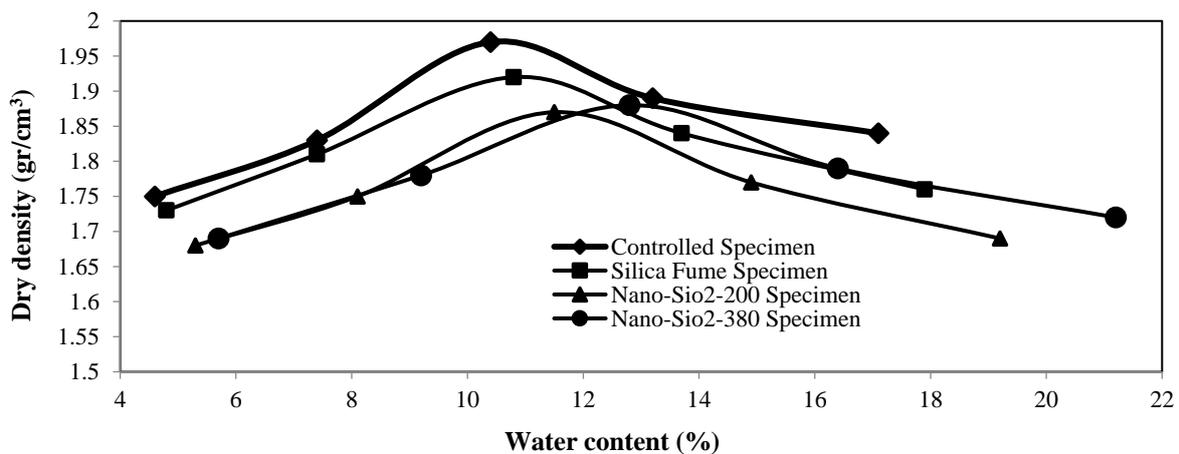
Fig. 6. The effects of type of silica material on the compaction properties
