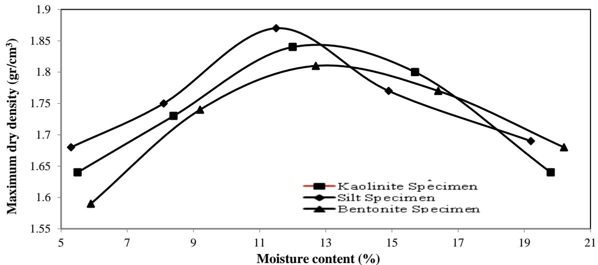
Fig. 5. Effect of type of fines on the dry density and optimum moisture content
