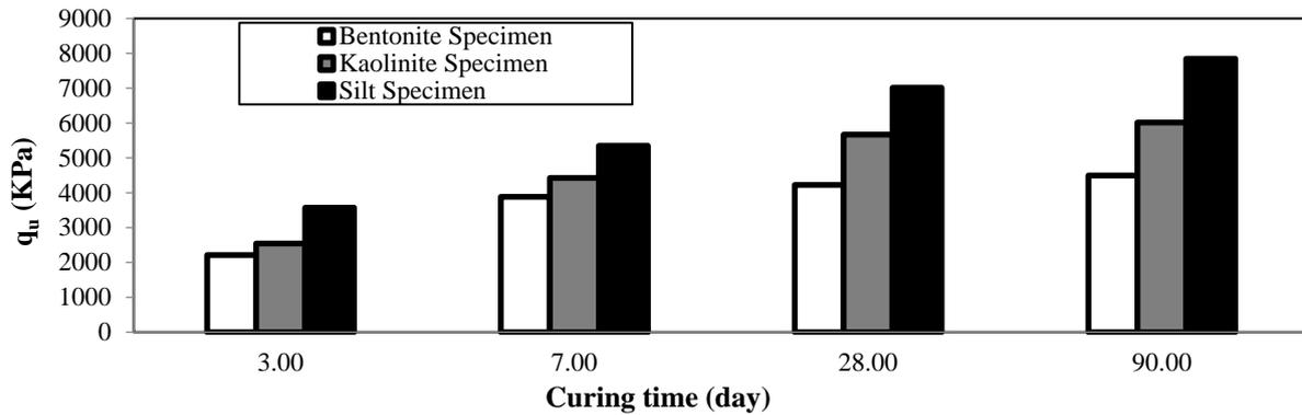
Fig. 9. The uniaxial compressive strength of soil-cement mixtures with different types of fines
