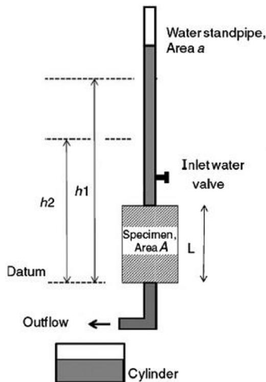
Fig. 3. Schematic of a variable head permeability test equipment (Tajdini et al., 2018)
