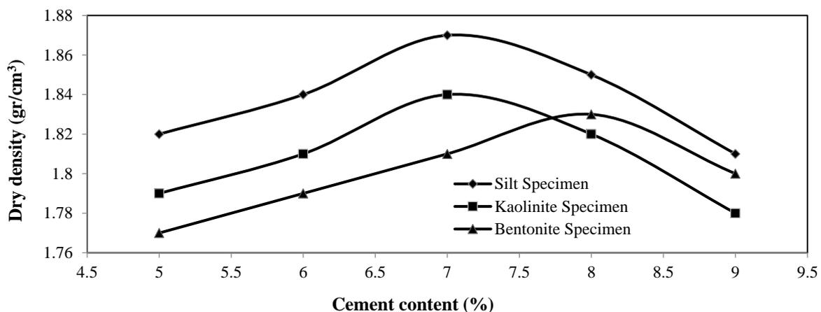
Fig. 4. Effect of cement content on the maximum dry density of the mixtures with different types of fines
