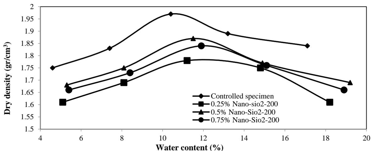
Fig. 7. The effect of nanosilica 200 content on the dry density and optimum moisture content
