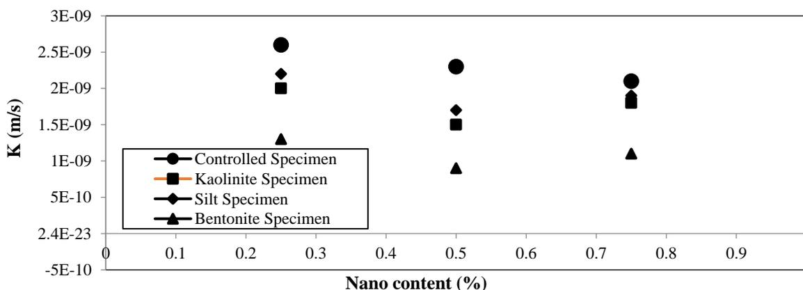
Fig. 12. Permeability of the mixtures with different types of fines
