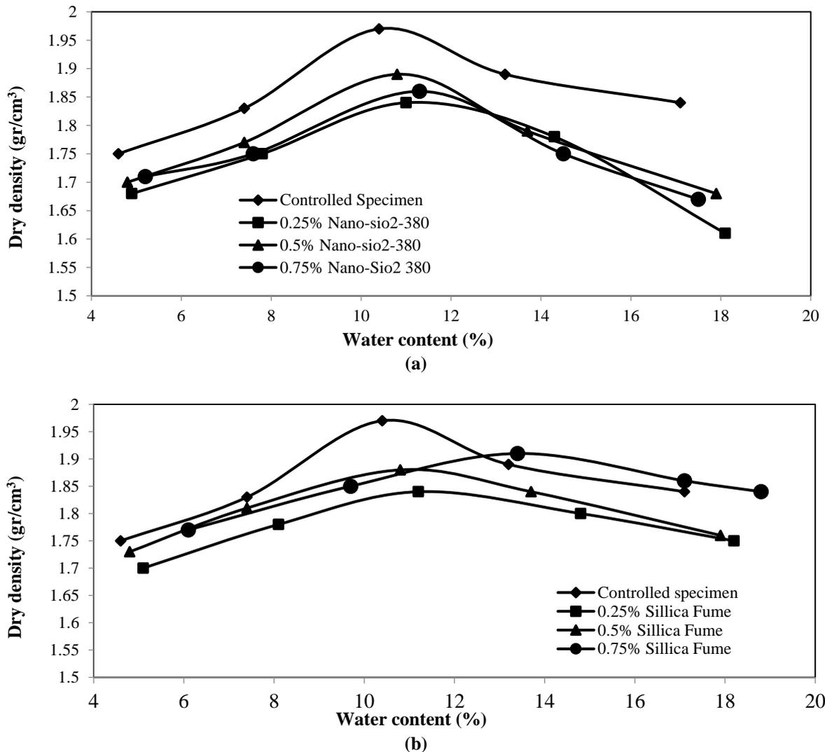
**Fig. 8.** The effects silica fume and nanosilica 380 on the dry density and optimum moisture content: a) Compaction curves of the mixtures containing microsilica and; b) Compaction curves of the mixtures containing nanosilica 380
