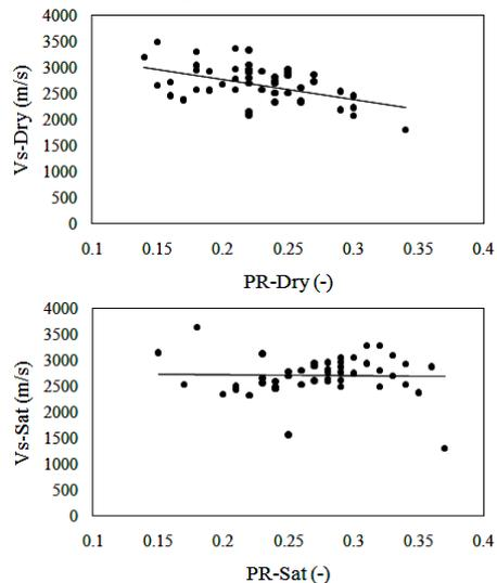
Fig. 11. The relationship between shear wave velocity and Poisson's ratio in dry and saturated conditions.
