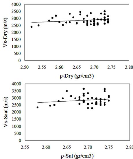
**Fig. 5.** The relationship between shear wave velocity and density in dry and saturated conditions.
