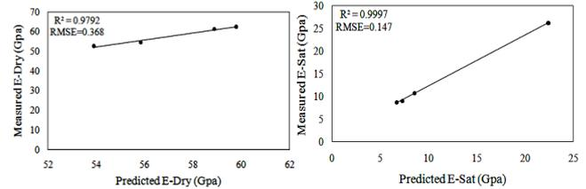
**Fig. 16.** Comparison of the measured and predicted moduli of elasticity in dry and saturated conditions.
