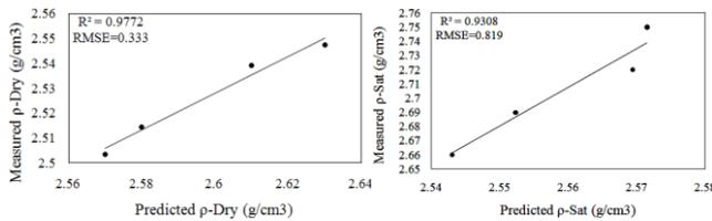
**Fig. 12.** Comparison of the measured and predicted density values in dry and saturated conditions.
