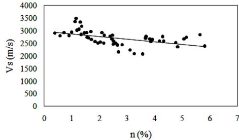
**Fig. 7.** The relationship between shear wave velocity and porosity.
