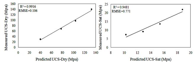
**Fig. 17.** Comparison of the measured and predicted unconfined compressive strengths in dry and saturated conditions.
