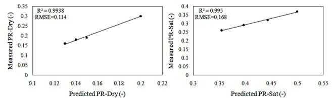
**Fig. 18.** Comparison of the measured and predicted dry Poisson's ratios.
