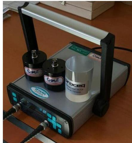
Fig. 4. The PUNDIT device used for  $V_s$  measurement.
