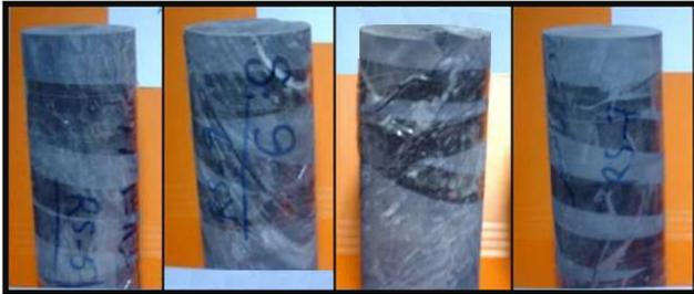
Fig. 3. The prepared core samples for conducting the laboratory tests.
