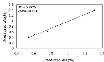
**Fig. 13.** Comparison of the measured and predicted water absorption values.
