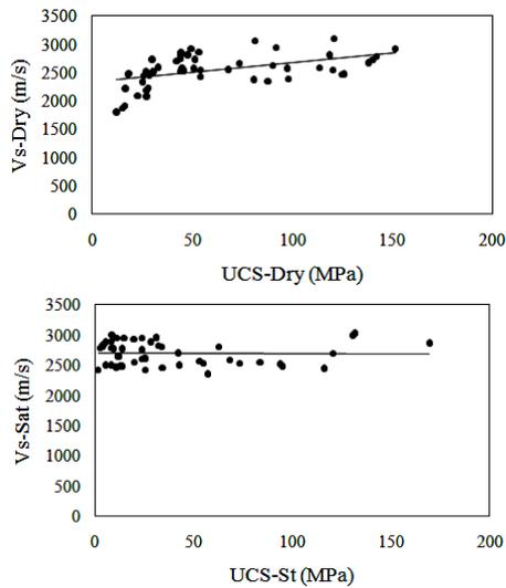
Fig. 10. The relationship between shear wave velocity and unconfined compressive strength in dry and saturated conditions.
