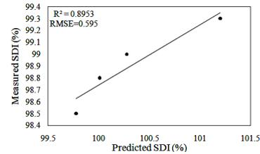
**Fig. 15.** Comparison of the measured and predicted slake durability index values.
