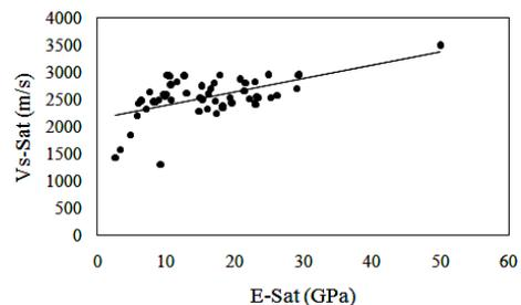
**Fig. 9.** The relationship between shear wave velocity and modulus of elasticity in dry and saturated conditions.
