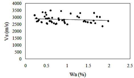
**Fig. 6.** The relationship between shear wave velocity and water absorption.
