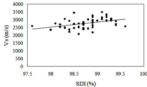
**Fig. 8.** The relationship between shear wave velocity and slake durability index.
